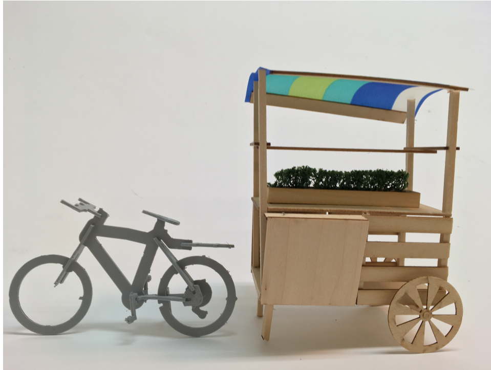
A scale model mock-up made from laser cut birch. At the time this model was created, it was approaching the final design to be used for full scale fabrication. Source: Teo Willard
