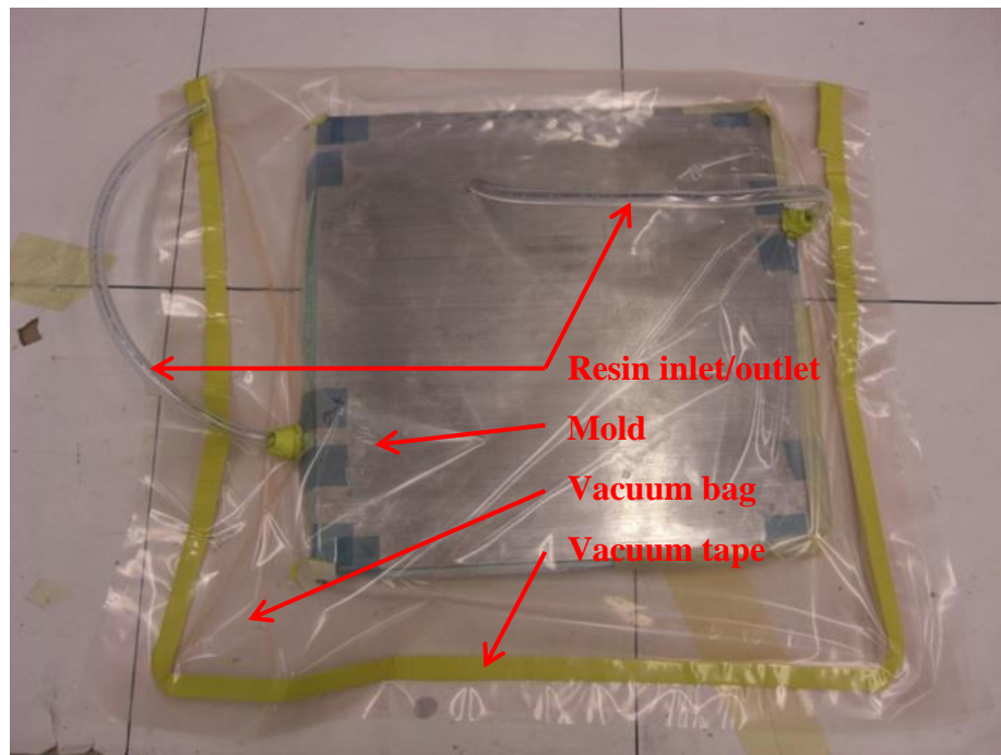
Figure 2.3: VARTM bagged and sealed infusion mold
