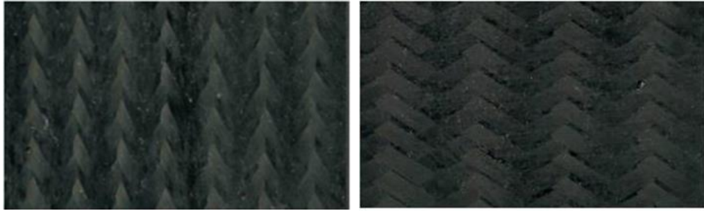
Figure 1.2: Cured TBC 30 material (left) and TBC 60 material (right)
