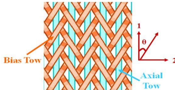
Figure 1.1: Diagram of 2D triaxially braided textile
