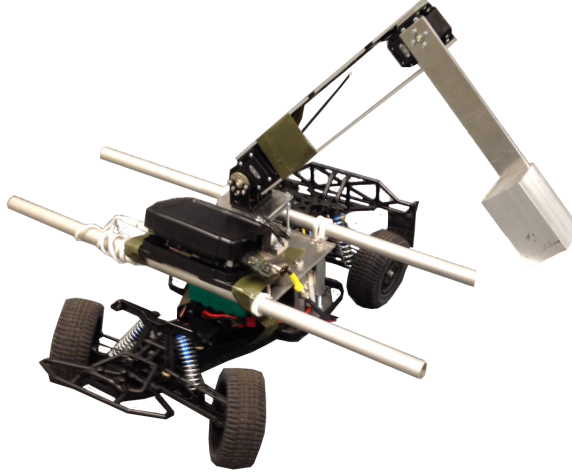
Figure 3.4: Modified 1:10 scale RC car with a two-link manipulator arm used for experimental validation.
