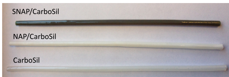
Figure 3.2. The images of SNAP-doped (top), NAP-doped (middle) and plain control CarboSil catheters, all with blank CarboSil topcoats.
