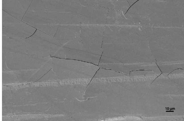
Figure A.3: SEM image of a cracked FeOOH on WO 3 . The pictured film was synthesized using longer deposition times, generating a thicker layer. Cracking in the film was observed due to the film drying out.
