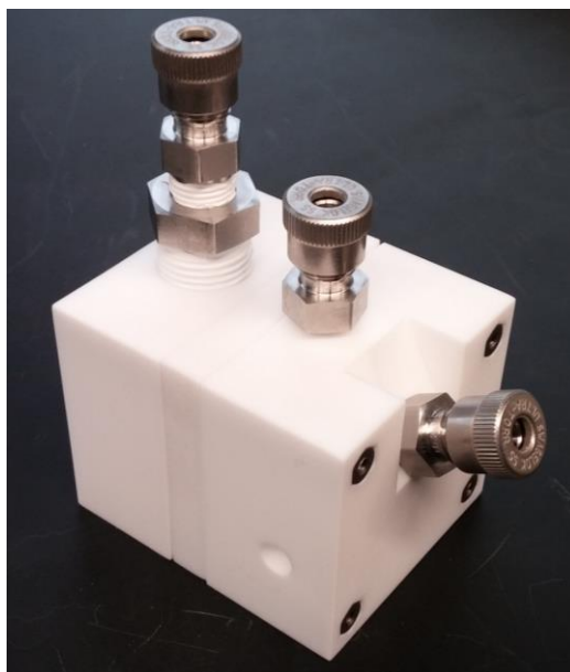
Figure 4.2.3-3 Assembled Bulk Electrolysis cell.
