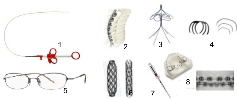
Figure 1.6: Examples of NiTi applications utilizing superelasticity: 1. endoscopy tools, 2. spinal implants, 3. vena cava filters, 4. NiTi clips, 5. glass frames, 6. arterial stents, 7. surgical files, 8. orthodontics arch wires. [39], [40], [89]
