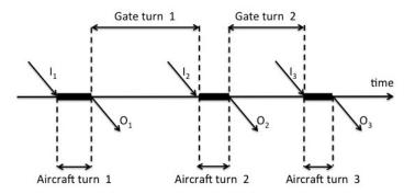
Figure 2.1: Gate schedule with three aircraft turns and two gate turns
