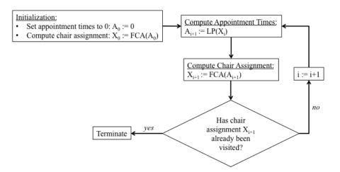
Figure 3.3: Representation of the algorithm
