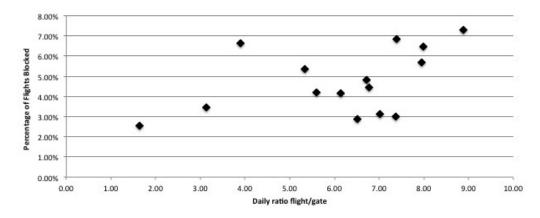
Figure 2.8: Percentage of flights blocked in each station as a function of the daily number of flights per gate in Period 3
