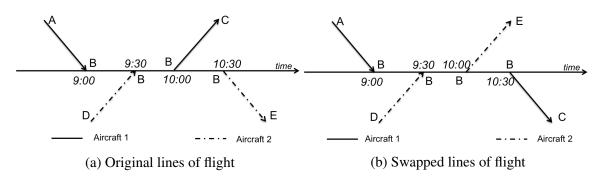
Figure 5.3: Example of swapped flights between two aircraft
