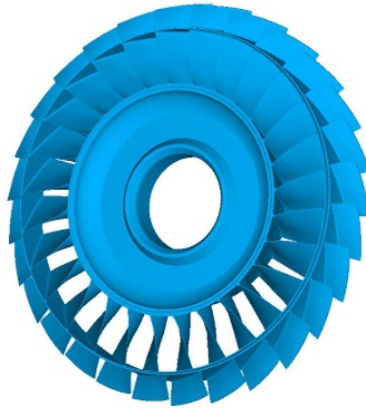
Figure 2.1: A finite element model of the FLADE™system
