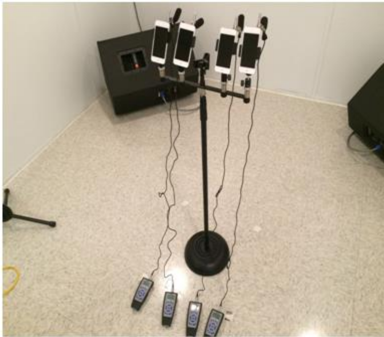
Figure 3-1 The paired dosimeters and devices mounted on a stand in the reverberant sound chamber prior to testing in experiment 1
