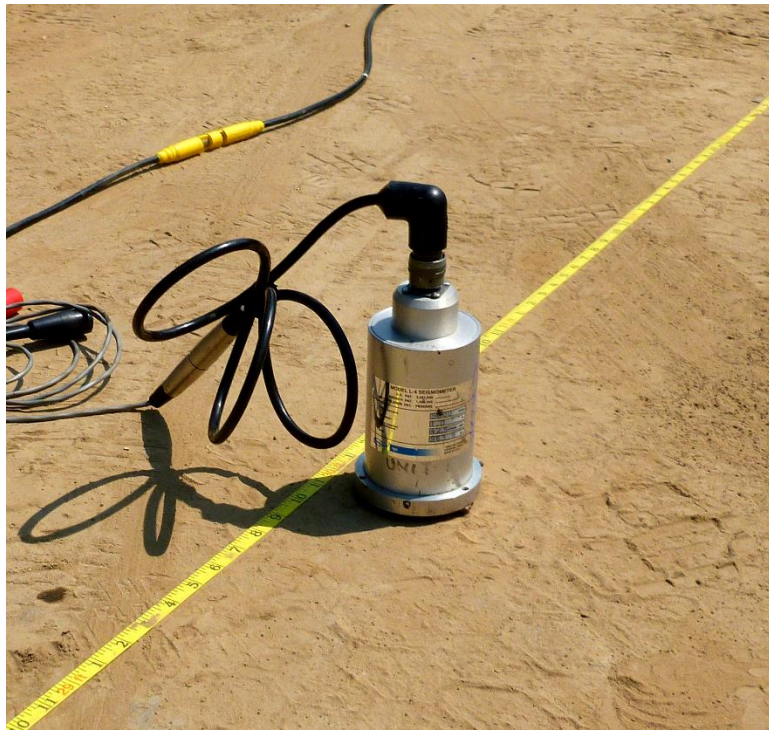
Figure 5-2 Vertical seismometer used to measure surface ground motions
