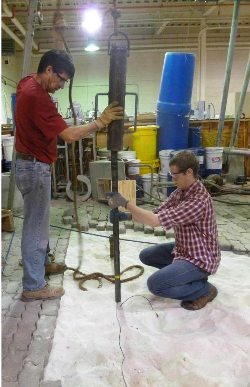
Figure 8-18 Pushing a sensor package to the desired depth in the sand bin
