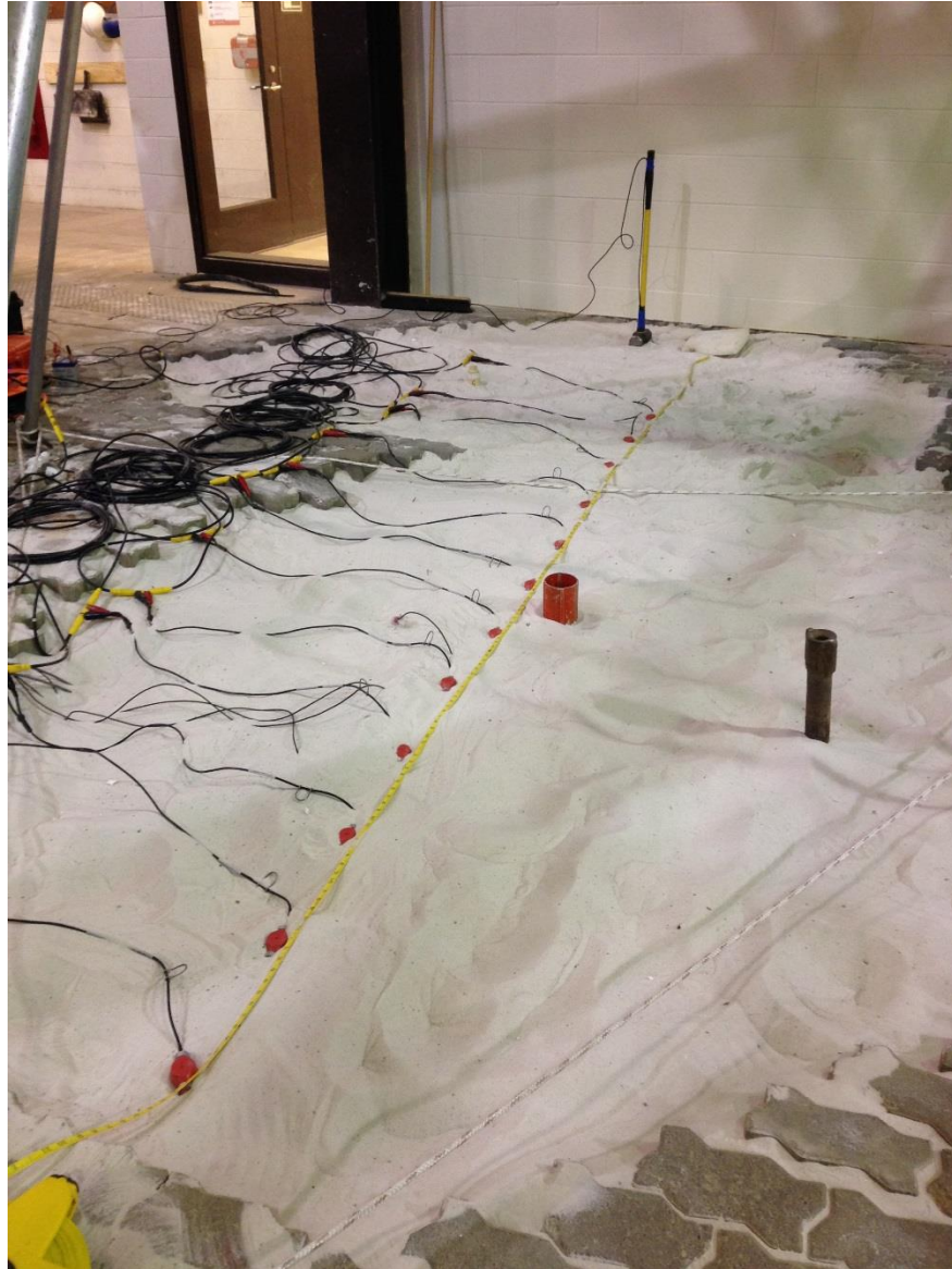
Figure 8-11 Configuration of the MASW testing in the sand bin
