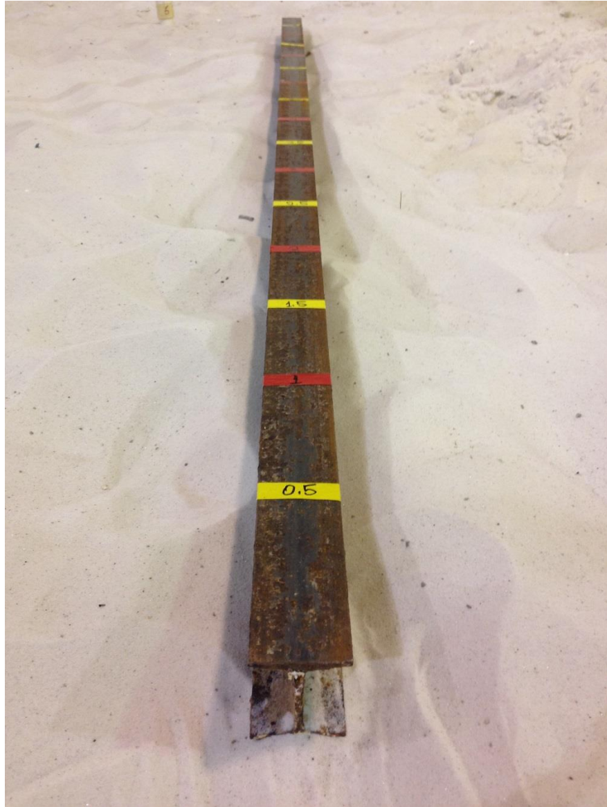
Figure 8-13 View of S 3x5.7 section
