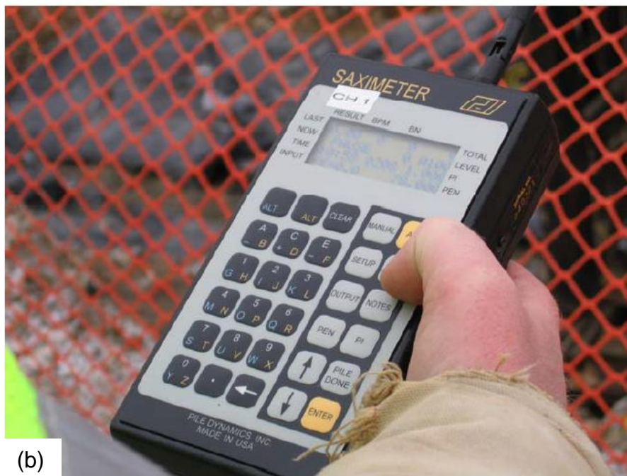
Figure 4-14 (a) Proximity switches and transmitter attached on diesel hammer and (b) E-Saximeter wireless device (from Hannigan 2006)
