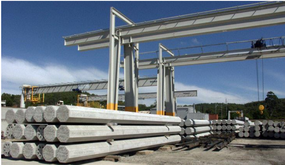
Figure 4-2 Precast concrete piles (Courtesy of Structural Concrete Industries)
