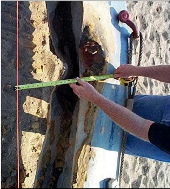
Figure 4-27 Extracted H-pile after PDA damage indication (from Hannigan 2006)
