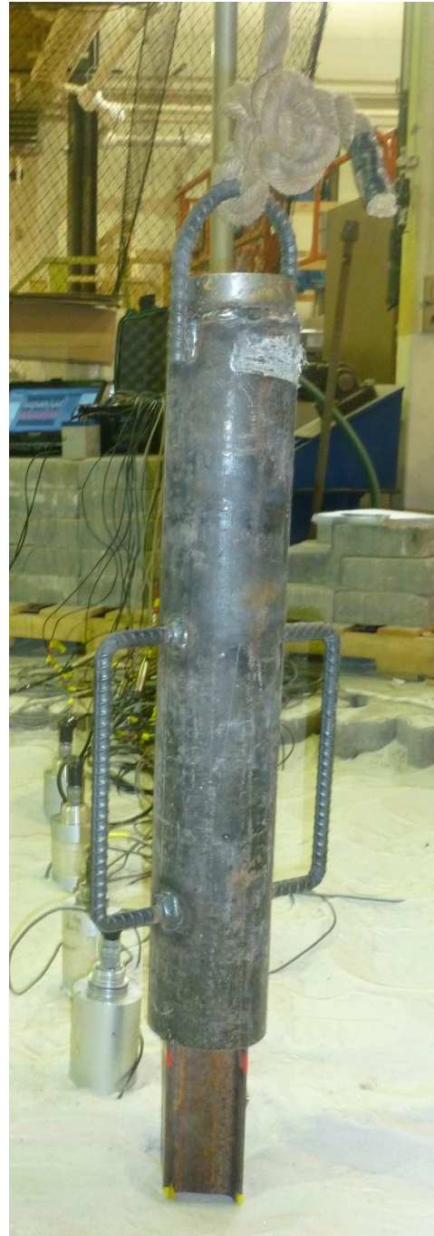
Figure 8-14 Cross section and view of fence post driver used to drive the pile in the sand bin (not to scale)
