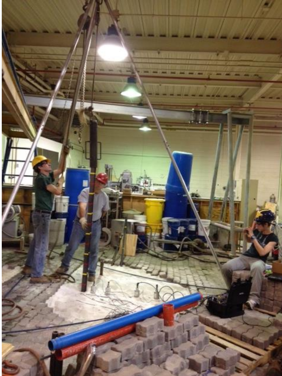
Figure 8-15 Driving of the pile in the sand bin using the tripod system
