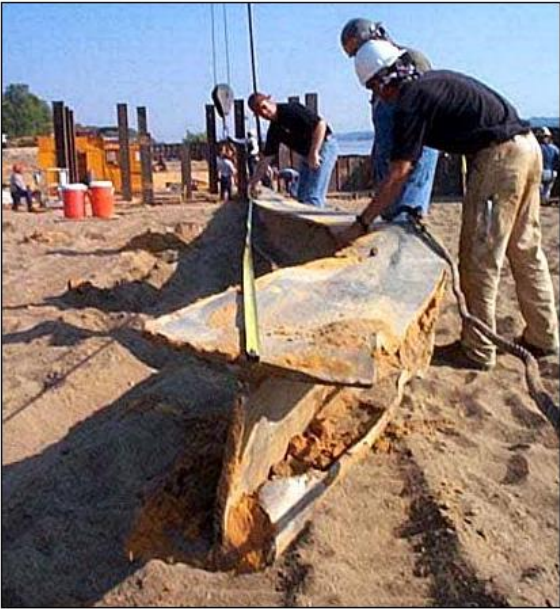
Figure 4-27 Extracted H-pile after PDA damage indication (from Hannigan 2006)
