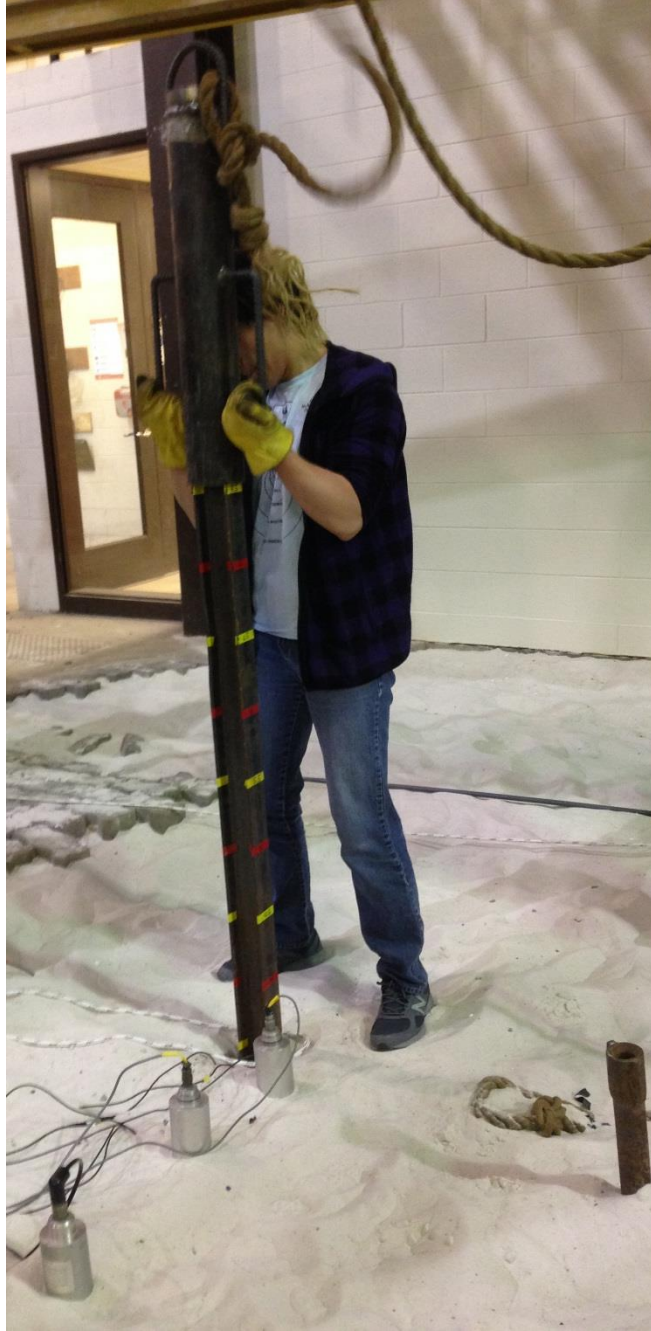
Figure 8-16 Driving the pile by lifting the driver by its handles
