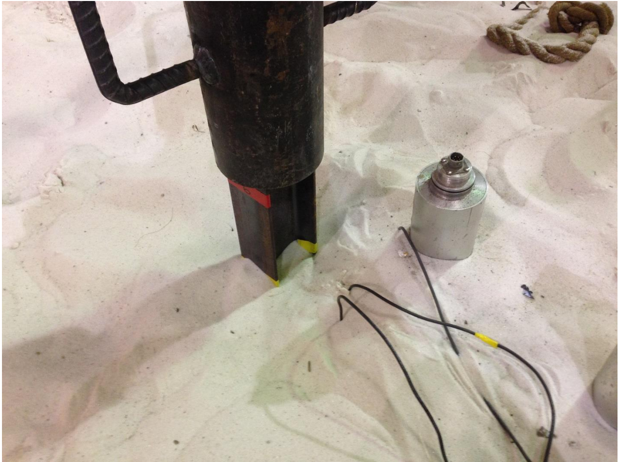
Figure 8-22 Pile, driver and wires of closest buried sensors on the ground surface
