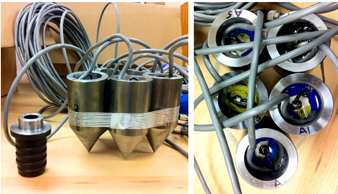
Figure 5-9 Sensor casings and rod to cone adaptor
