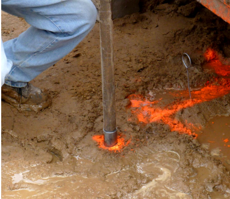
Figure 5-14 Rod and cone positioning on the ground surface
