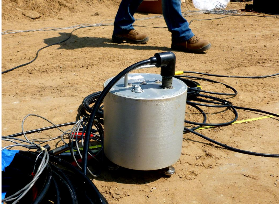
Figure 5-1 Triaxial seismometer used to measure surface ground motions
