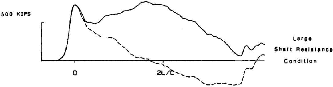
Figure 4-26 Force and velocity wave traces for large shaft resistance condition (from Hannigan 1990)
