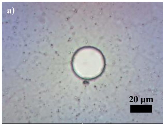
Figure 5.9 a) Optical image and b) scanning electron image of 30 μm diameter pinhole SU-8 pattern.
