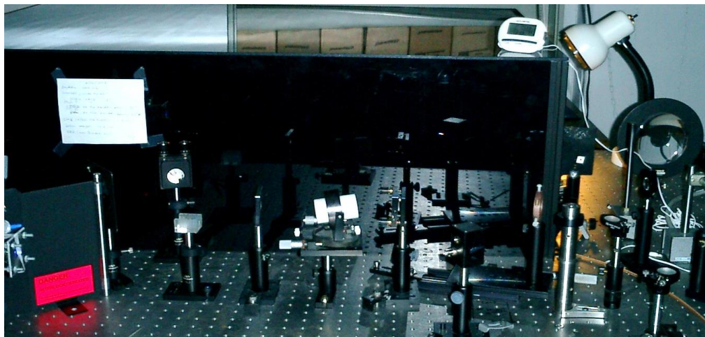
Figure 5-27 Image of the time-correlated single photon counting set up.
