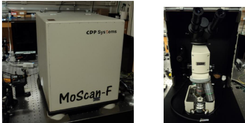
Figure 5-20 Image of the MoScan NSOM microscope enclosure (left), the optical and inverted microscope (right) for NSOM collection.
