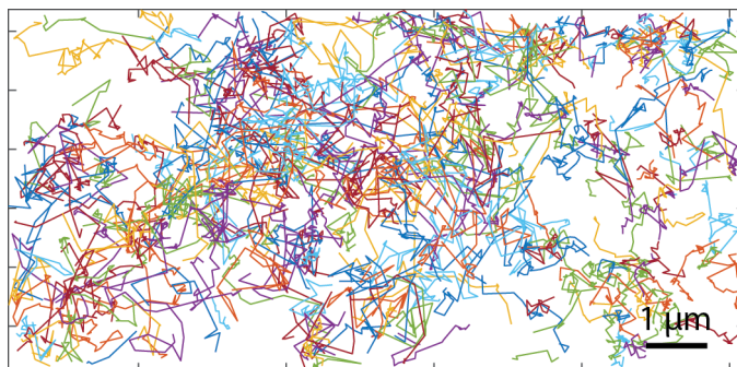
Figure 4.3.6: 1-palmitoyl-2-oleoyl- sn -glycero-3-phosphocholine (POPC, Avanti) and the lipid dye DiI C12 (ThermoFisher) were mixed together in chloroform at final concentrations of 5 \text{ mg mL}^{-1} and 1 : 4 \times 10^{-5} from stock concentration, respectively. 1.5 wt% agarose and then 30 \mu\text{L} of lipid/dye solution were spin coated onto a coverslip at 5000 rpm. 30 \mu\text{L} PBS was then placed on top of the dried lipids and a top coverslip was then added. The sparse DiI was imaged with a 561 nm fluorescence excitation laser (Coherent Sapphire 560-50) with a power density of 0.01 \text{ mW } \mu\text{m}^{-2} . The sample was imaged on a Photometrics Evolve EMCCD camera and the diffusing DiI was then localized and tracked. Shown here are the 336 trajectories used in the analysis shown in Figures 4.3.7 and 4.3.8.
