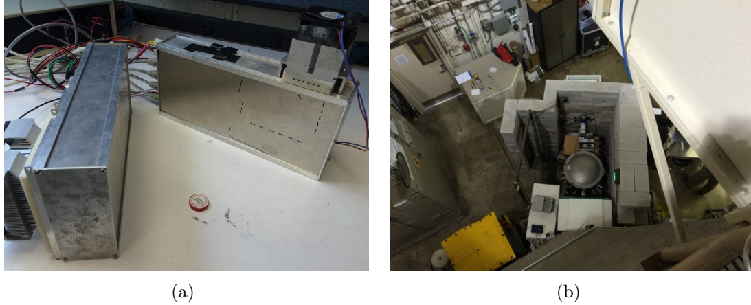
Figure 4.1: (a) Polaris SP system with both plane's cathodes facing a button source of gamma rays. (b) Output of the beam port at the NARS laboratory. The beam was incident from the bottom of the picture, through the round sample chamber, and onto the cathodes of Polaris SP's plane B, positioned near the center of the photograph.
