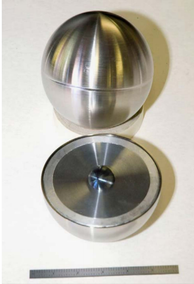
Figure 7.11: Photograph of two RSTDs [12]. One has top hemisphere removed, revealing its DU core at center. The outer layer consists of an Al-HEU alloy enclosed in a thin Al shell.
