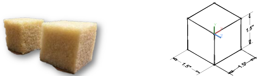
Figure 6.6 Picture of the PU Foam Cube and Schematic with Dimensions
