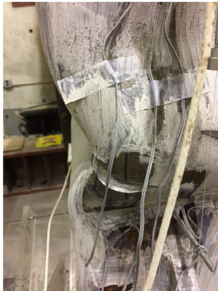
Figure 4.23 Local Buckling of Collar Connection with Stiffeners at the First 0.06 rad. Cycle
