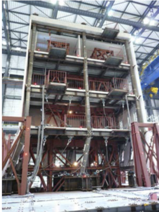
Figure 1.1 First Story Collapse Mechanism of the Steel Moment Frame (Lignos et al., 2013)
