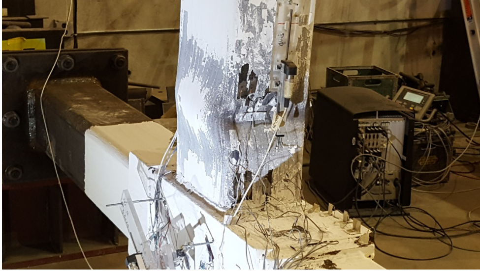
Figure 4.19 Local Buckling of Collar Connection without Stiffeners at the First Cycle of 0.06 rad. Rotation Cycle
