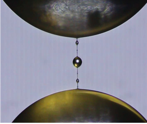
Figure 1.2: An elongated saliva filament after an imposed axial step-strain in a capillary break-up rheometry experiment forms a thin filament with beads-on-a-string.
