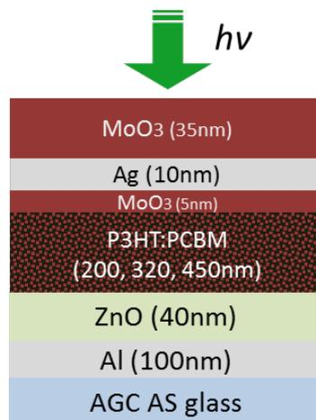
**Figure 2.1** Device structure of the inverted OPD with top illumination. The thickness for each layer indicates the optimized values for the fabricated OPD.
