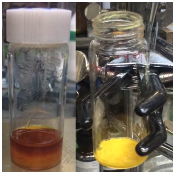
Figure S3. Pictures during recrystallization: (left) crude solution left at -30\text{ }^{\circ}\text{C} for overnight; (right) yellowish solids of 2 after quick pipetting out of solvent with precooled Pasteur pipette and washing twice with cold hexane. (If a saturated solution was used for recrystallization, it is very difficult to remove mother liquor. We recommend to use unsaturated solution for obtaining 2 with high purity.)
