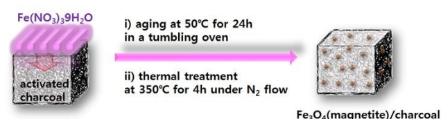
Scheme 1. A facile synthesis of \text{Fe}_3\text{O}_4/\text{C} nanocatalysts by infiltration
