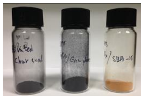
Figure 1. Pictorial representation of \text{Fe}_3\text{O}_4 NPs on charcoal, single-layer graphene, and SBA-15 from left to right.
