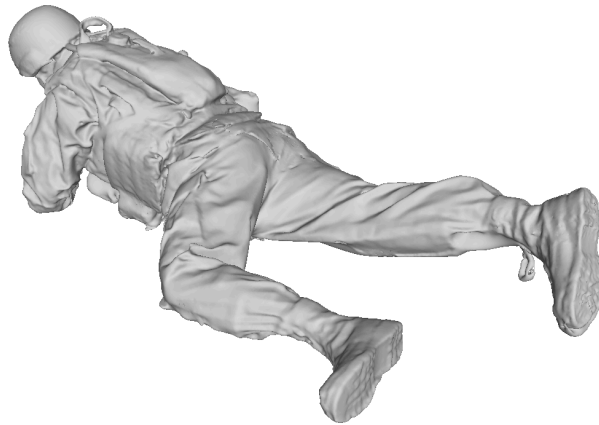
Figure 24. Sample data obtained from a prone volunteer using a transparent scanning surface.
