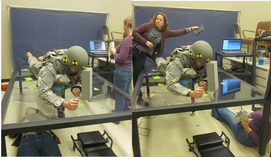
Figure 23. Using hand-held scanners to capture body shape in prone postures on a transparent table.
