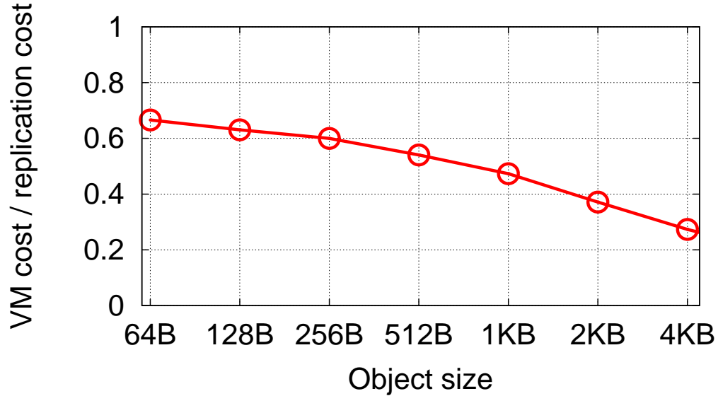
Figure 5.4: When reads/writes are relayed through VMs, fraction of cost accounted for by these VMs relative to total cost to execute reads and writes.
