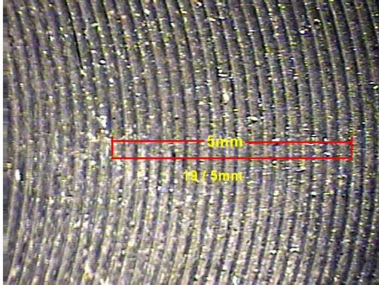
Figure 2.6: Banded structure of a friction stir welded Ti-6Al-4V sample, showing a band width about 0.23mm
