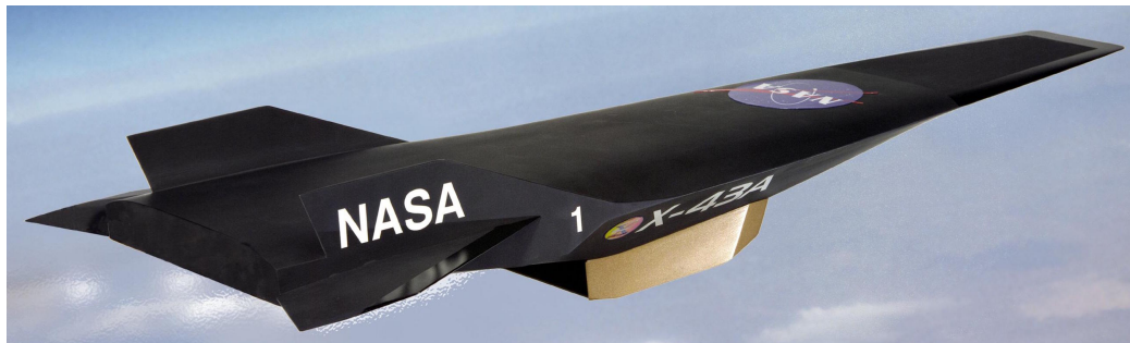
(c) X-43A : fastest jet-powered unmanned aircraft, which flew at Mach 9.68 (2004). Figure from NASA Illustrations.
