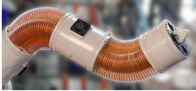
Figure 6.1: Bellows-driven continuum joints are used to create robots without finite degrees of freedom. Sensing the motion of such robots is a challenge. The inductance-based sensors presented in this work will bring estimation and control to robots like the one pictured here (created by Pneubotics).
