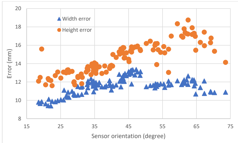
Figure 3-8: Error of dimensions with respect to sensor orientations for stairs.
