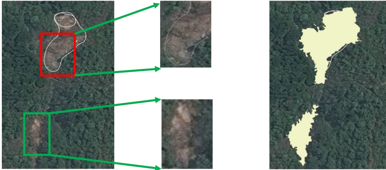
Figure 6-4: Example of similar visual appearance of landslide and ground.
