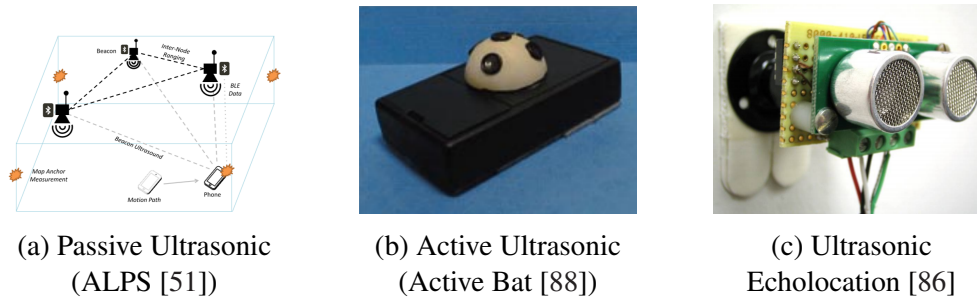
Figure 2.4: Acoustic Localization Methodologies. Localization technologies utilizing acoustic techniques have been gaining popularity due to the prevalence of acoustic transducers in smartphones. Various techniques have been proposed including near-ultrasonic geopositioning with time-of-flight to echolocation approaches which calculate position based on the expected echo “fingerprint” of the surrounding environment. However, tag cost and the coverage afforded by these acoustic approaches have limited their applicability.
