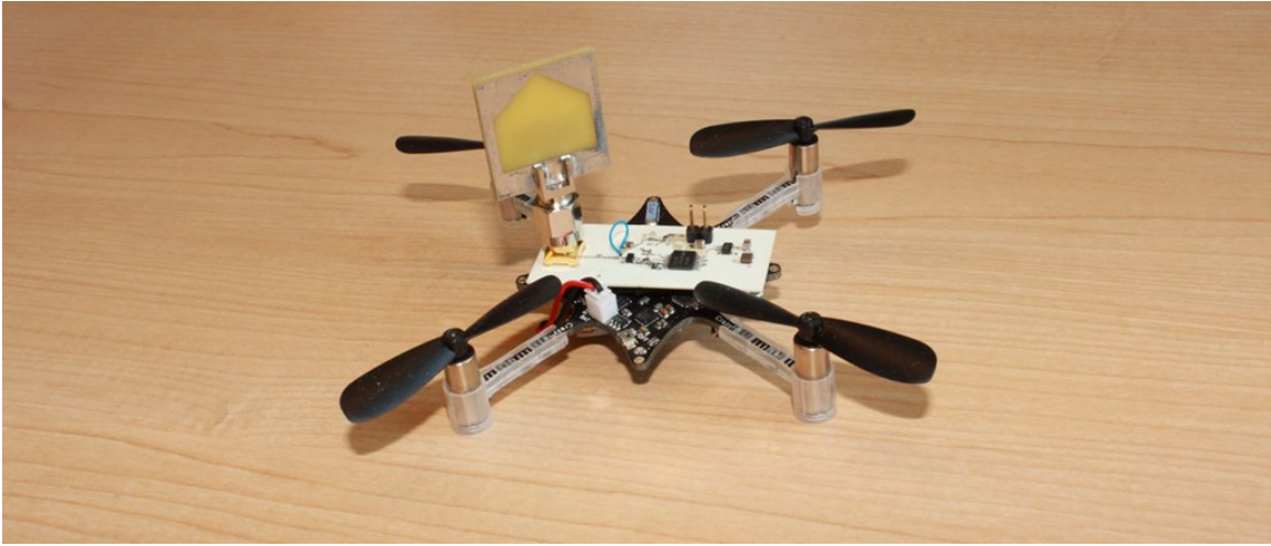
Figure 4.7: A Harmonium Tag on a Micro Quadrotor. This device has a maximum payload of 10 g and has only a 170 mAh battery. The Harmonium tag mass (3 g), volume ( 2.3 \text{ cm}^3 ), and power requirements (75 mW) are low enough to provide high-fidelity localization even for this constrained device. This enables real-time (19 Hz) location updates from a flying micro quadrotor.
