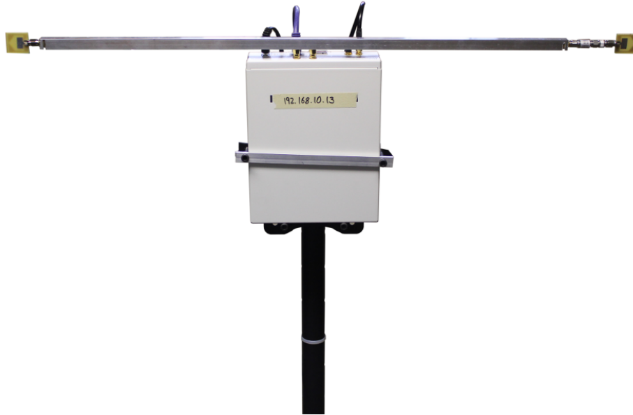
Figure 5.8: Slocalization Anchor Realization. The Slocalization anchor uses a commercial off-the-shelf Ettus USRP N210 software-defined radio with the SBX 400-4400 MHz daughterboard. Set up as a bistatic measurement, each anchor transmits and receives at different frequencies. Through bandstitching, a highly accurate measurement of the UWB channel impulse response is derived, allowing for an accurate determination of the backscatter tag’s CIR through time-domain correlation.
