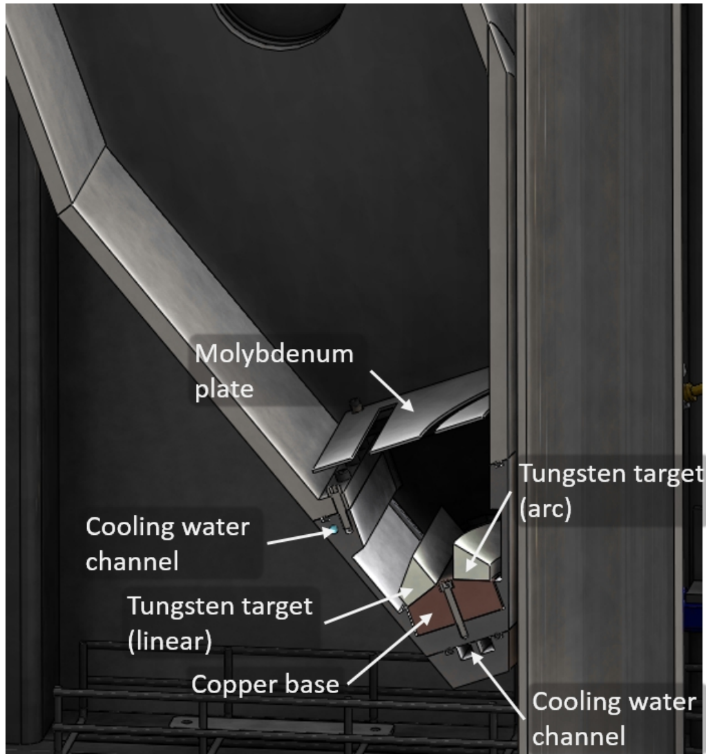
Figure 2.4: Cutout showing the bottom part of the chamber with the molybdenum safety screen, tungsten targets, and the water-cooled copper base. Note that the aluminum is also cooled underneath the o-ring to prevent o-ring failure. This system has two tungsten targets, linear and arc. The linear target was included simply to enable testing of the damage threshold of the tungsten material during the safety testing to generate the X-rays, and for other testing of basic ideas.
