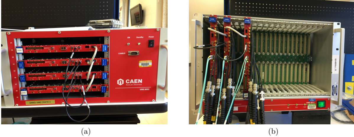
Figure 2.7: Digitizer configurations for the DPI using the CAEN V1720s (a) and CAEN V1730s (b).
