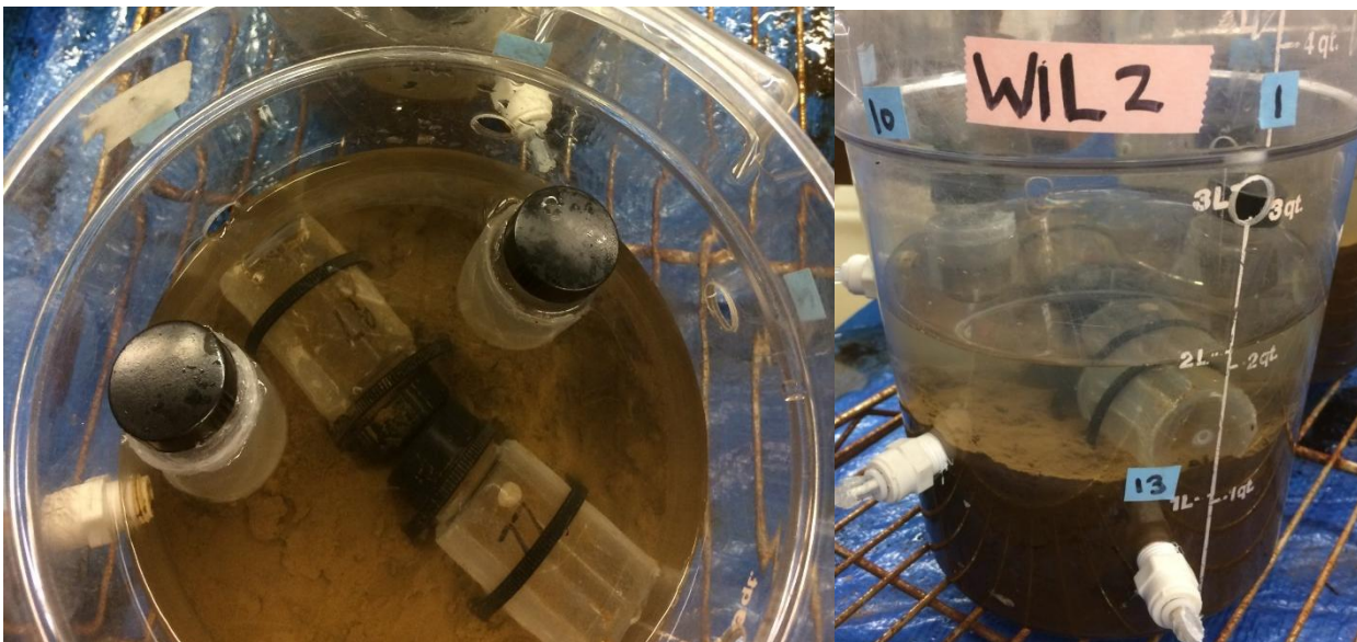
Figure 3-1. Organism exposure bottles depicted, where vertical bottles are for surface water exposure of D. magna and horizontally placed bottles are for sediment exposure of H. azteca .
