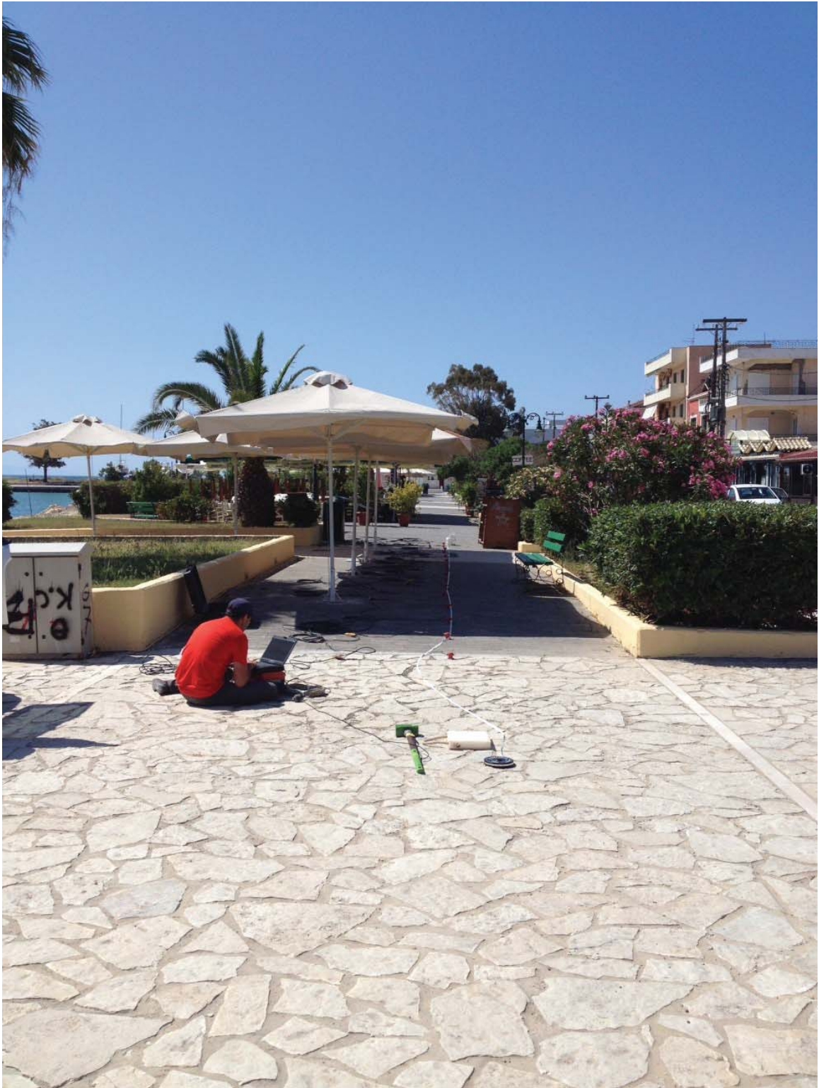
Figure 6.31: MASW setup for V_S measurements at Location 2
