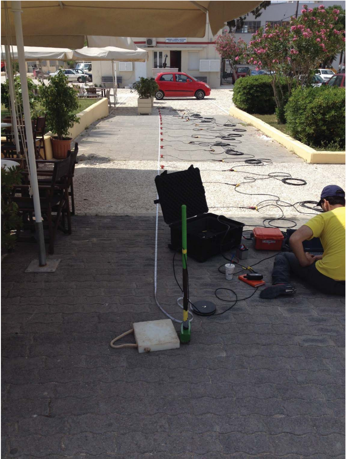
Figure 6.28: MASW setup for V_S measurements at Location 1
