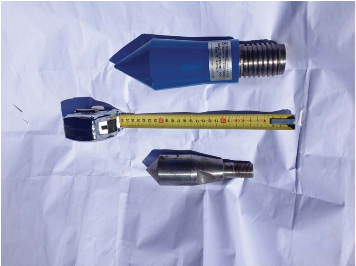
Figure 6.12: Larger Cone Tip (top) and Smaller Cone Tip (bottom)
