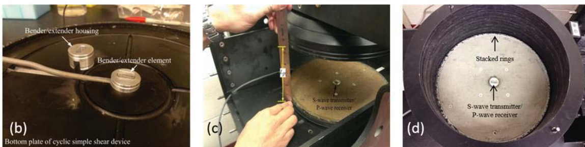
Figure 3.3: Bender element system (a) schematic, (b) housing units, (c) measurement of travel distance, and (d) placement of bender element in the bottom plate
