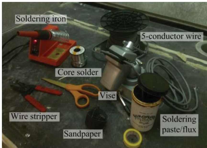
Figure 3.8: Tools and supplies to build the bender/extender elements (Sahadewa, unpublished)
