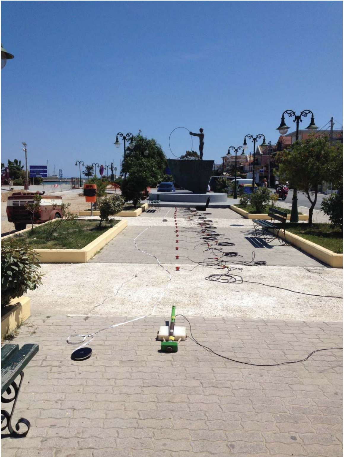
Figure 6.38: MASW setup for V_S measurements at Location 4
