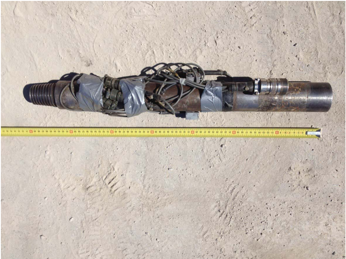
Figure 6.13: Instrumented rod used for energy measurements
