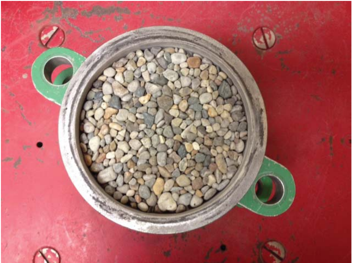
Figure 5.3: 60% Ottawa C109 Sand and 40% Pea Gravel after vibration table test
