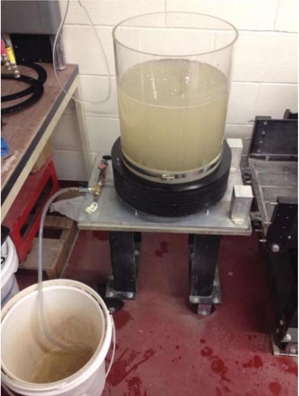
Figure 4.14: View of Specimen after sedimentation of Pea Gravel through 12" of water
