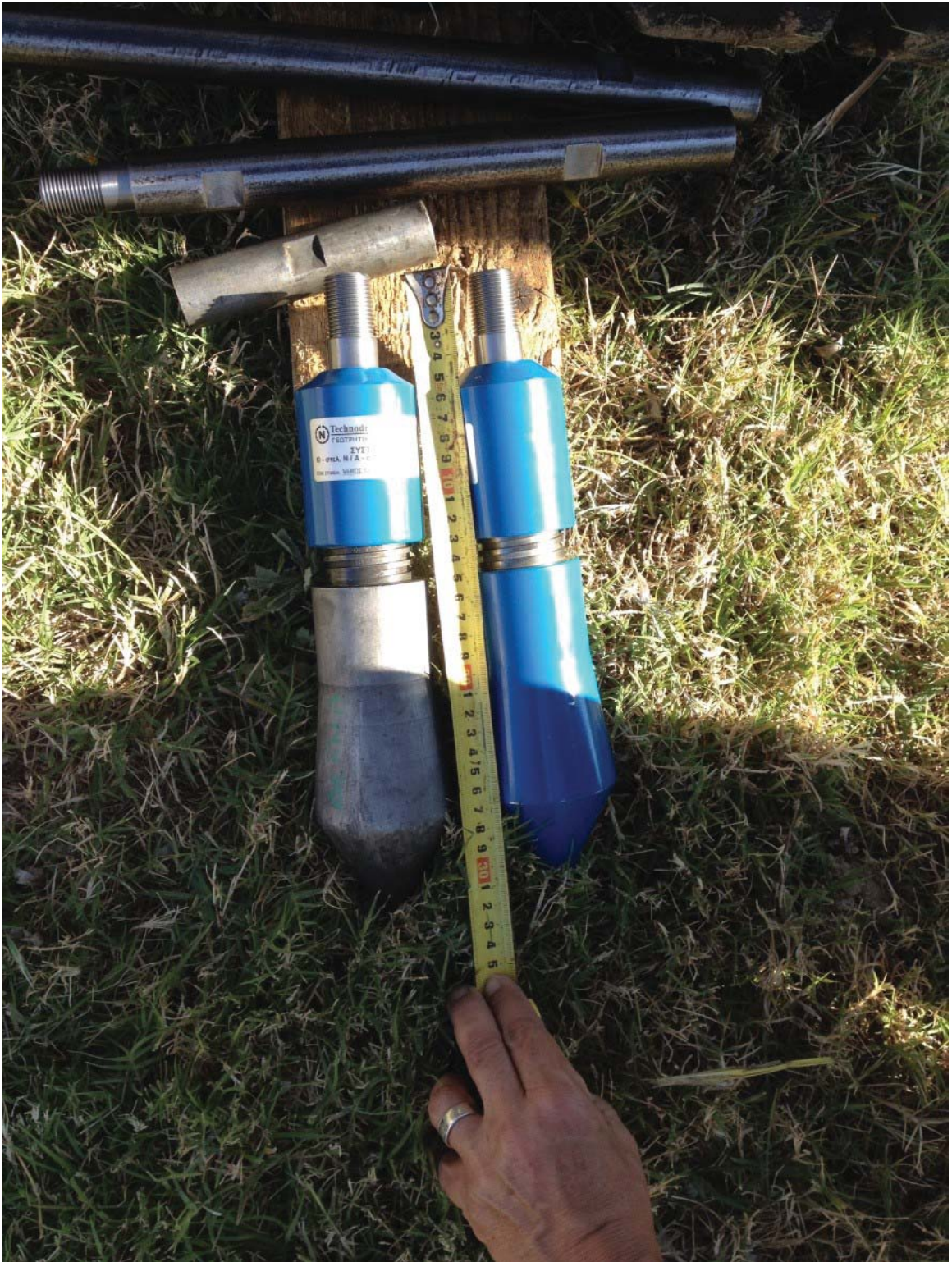
Figure 6.11: Cone Tips with adapters for connection to drill rods
