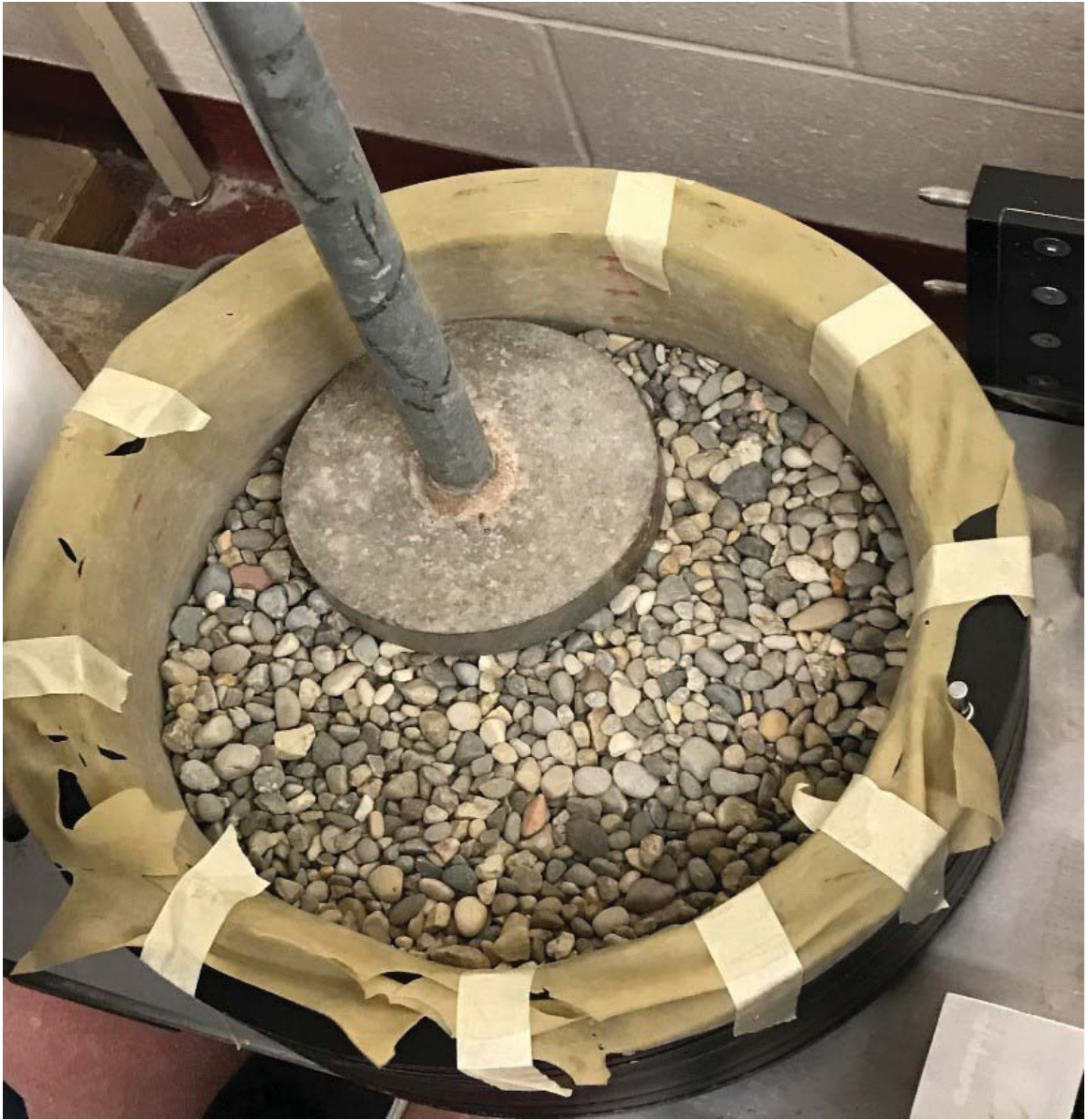
Figure 4.12: Example compaction of Pea Gravel in the dense state using drop weight
