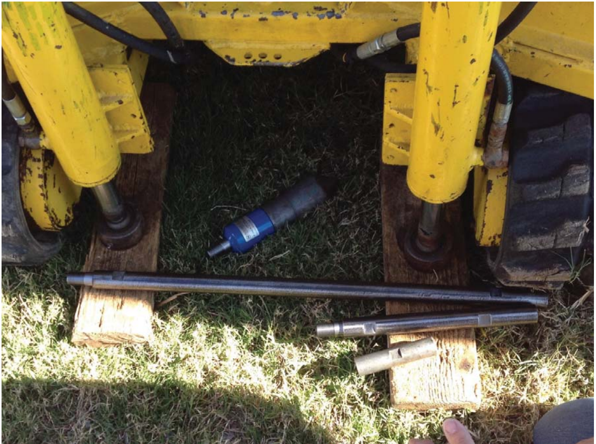
Figure 6.10: Cone Tip and rods used for DPT
