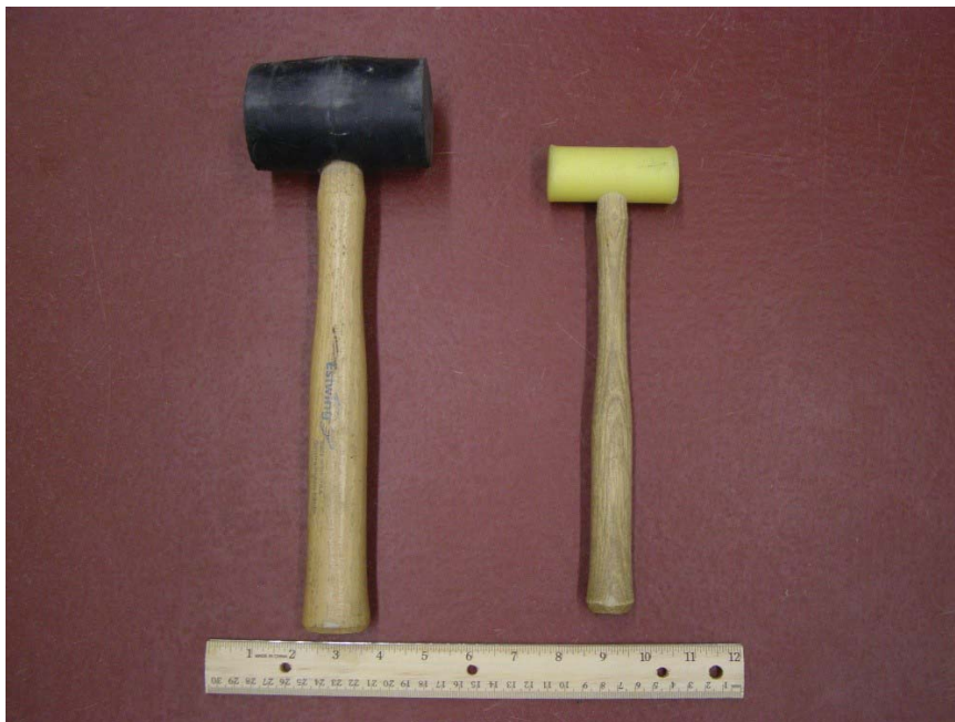
Figure 3.23: Rubber and Plastic Mallets used for impulse generation for accelerometers
