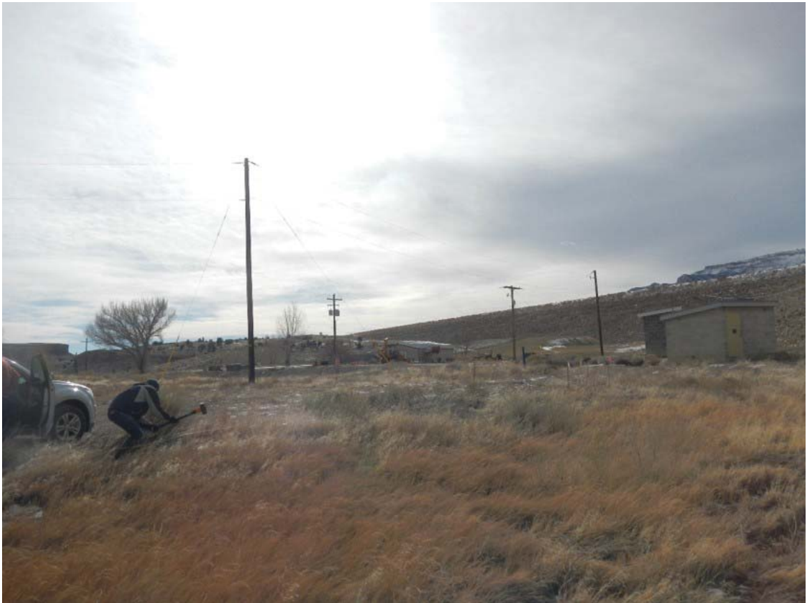
Figure 6.61: MASW setup for V_S measurements at Location 3 - Millsite Dam
