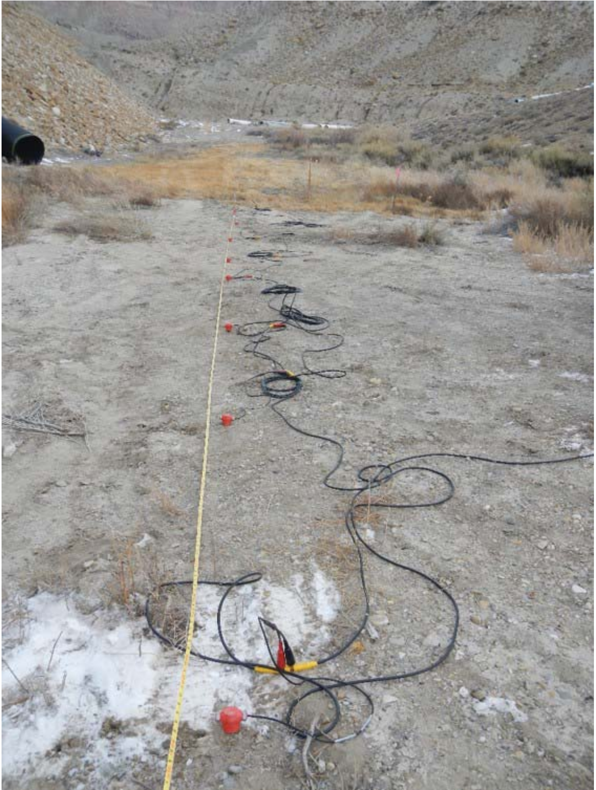
Figure 6.64: MASW setup for V_s measurements at Location 4 - Millsite Dam
