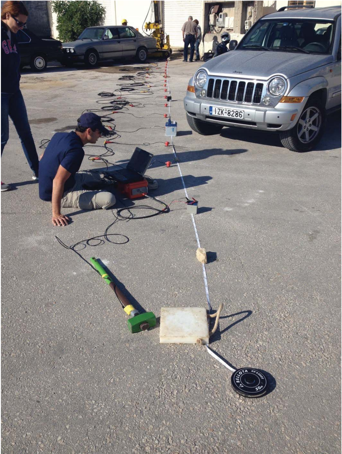
Figure 6.50: MASW setup for V_s measurements at Location 12
