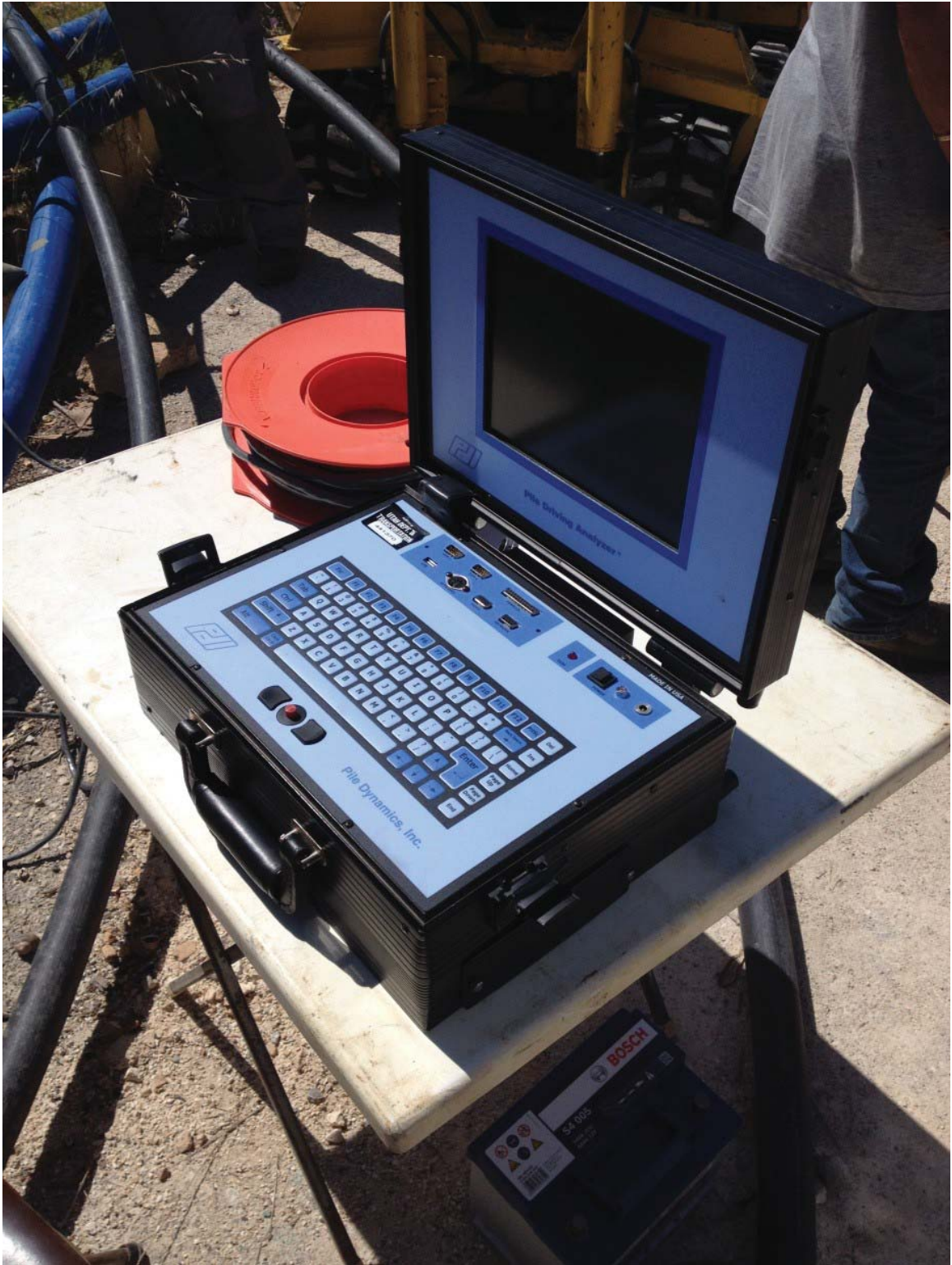
Figure 6.15: PDA energy measurement computer
