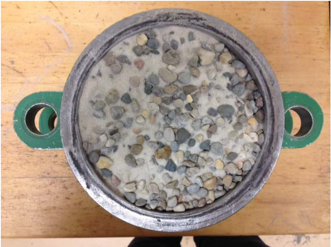
Figure 5.6: 40% Ottawa C109 Sand and 60% Pea Gravel after placement into mold
