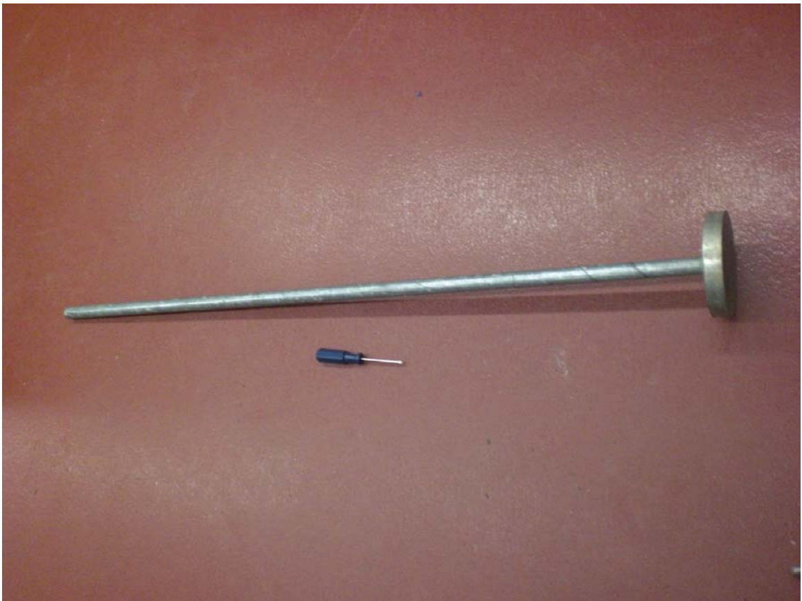
Figure 4.11: 5.5 kg drop weight used for preparation of dense specimens
