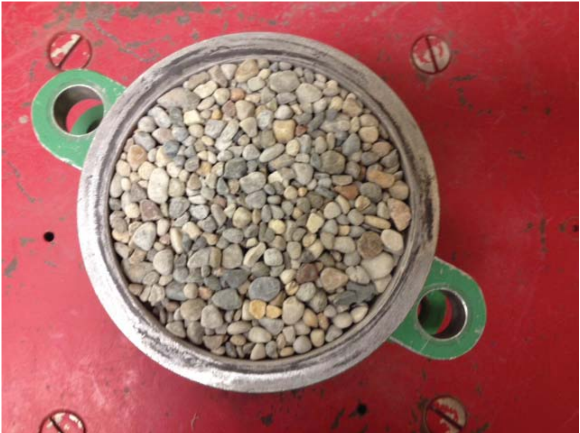
Figure 5.7: 40% Ottawa C109 Sand and 60% Pea Gravel after vibration table test
