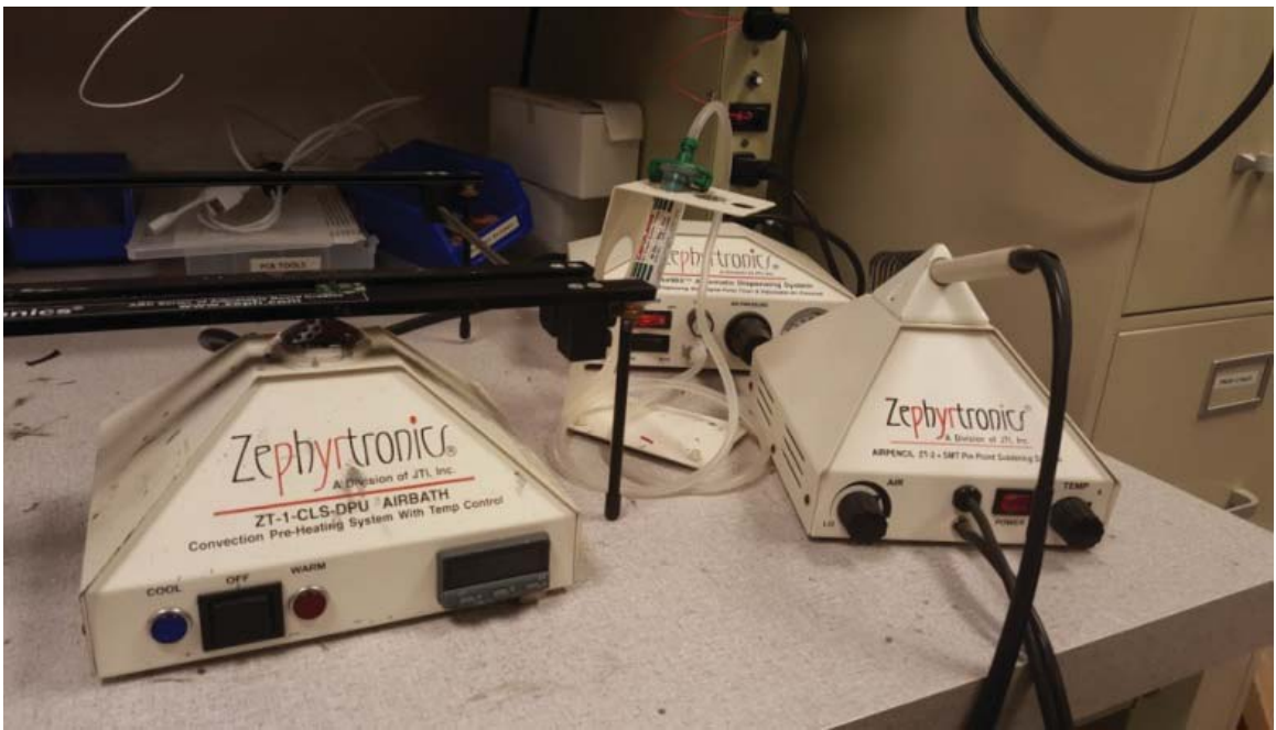
Figure 3.18: Tools used for replacement of capacitors on ADXL203EB
