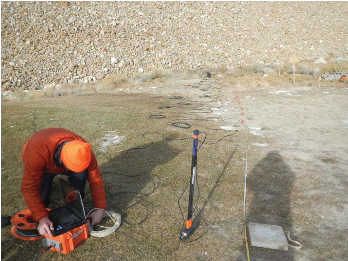
Figure 6.59: MASW setup for V_S measurements at Location 2 - Millsite Dam
