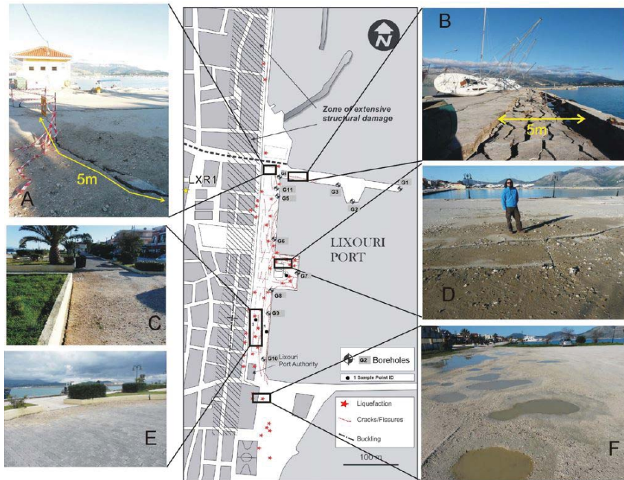
Figure 6.72: Location of Liquefaction observed in Lixouri following 2014 Cephalonia earthquakes (Papathanassiou et al. , 2016)
