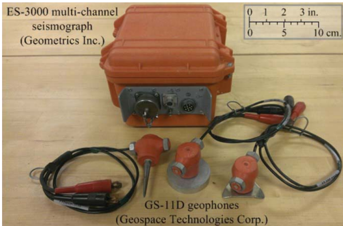
Figure 6.23: Seismograph and Geophones used in MASW testing ( Sahadewa, 2014 )
