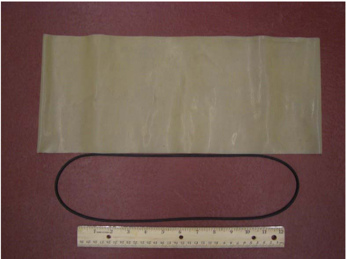
Figure 4.5: Membrane and O-ring for CSS device
