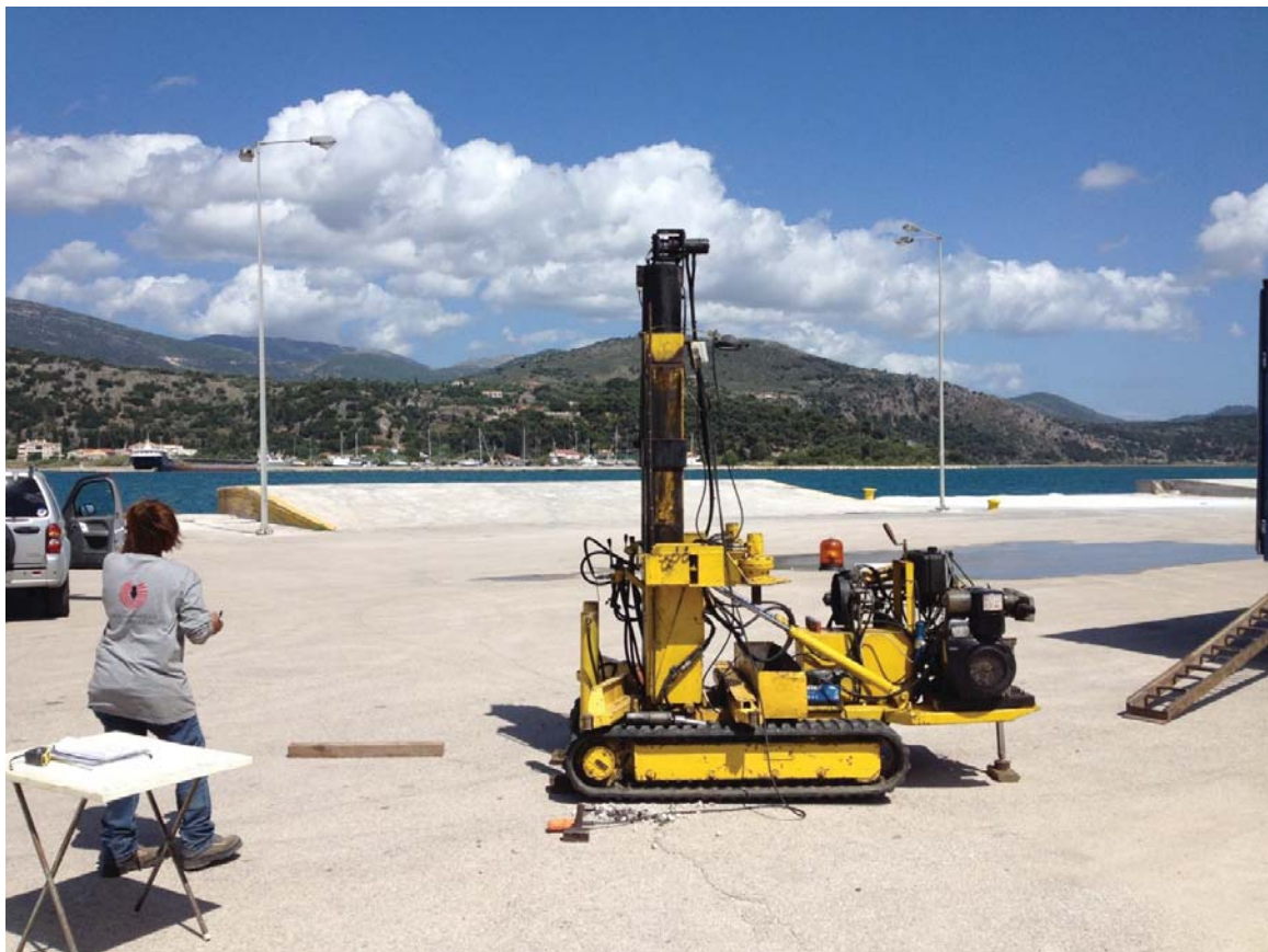
Figure 6.46: Setup of DPT at Location 11
