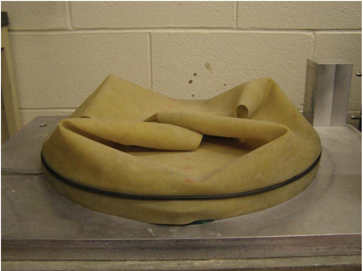
Figure 4.6: Placement of membrane and O-ring on bottom pedestal of baseplate
