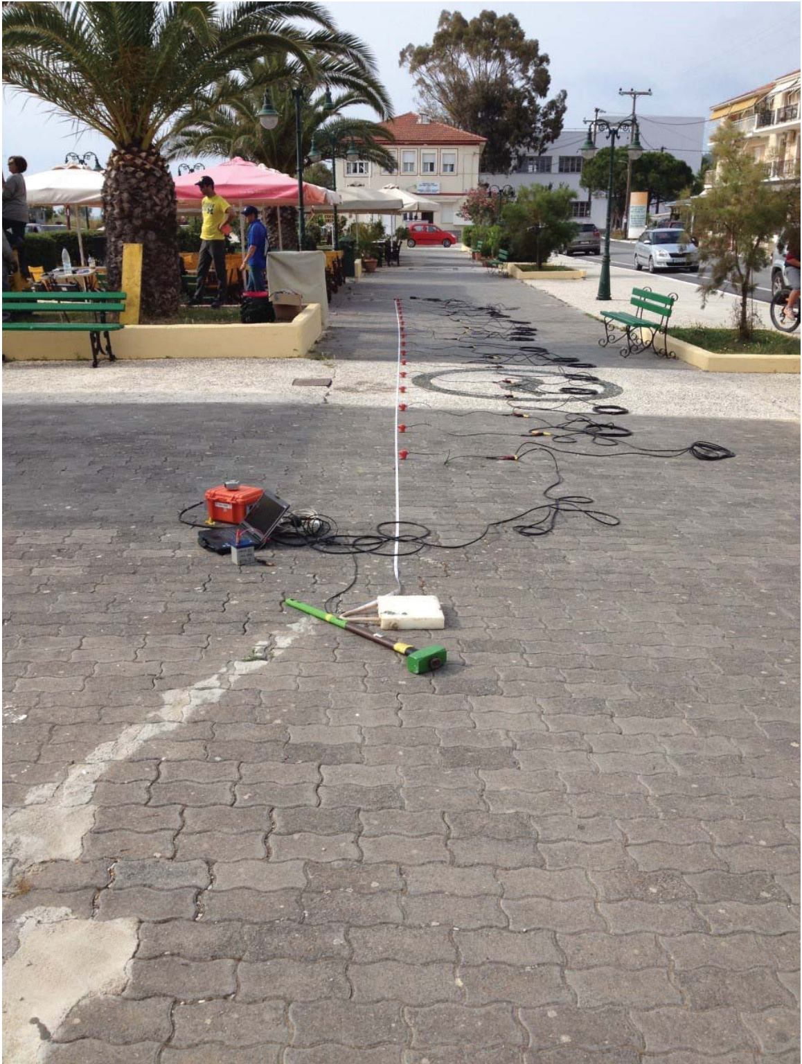
Figure 6.24: MASW setup with 1 m geophone spacing and 3 m hammer offset
