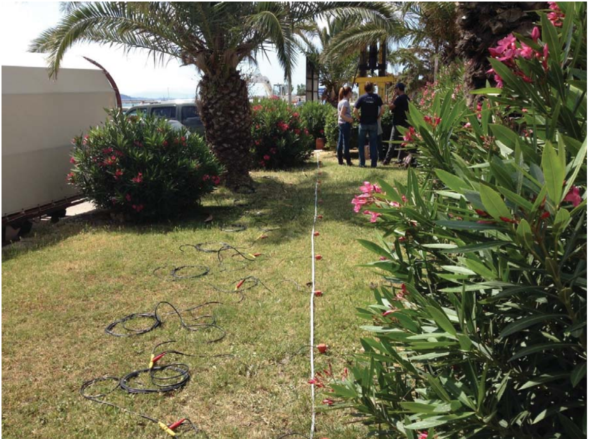
Figure 6.41: MASW setup for V_S measurements at Location 5
