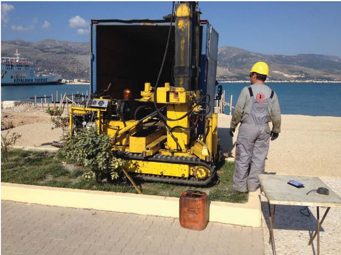
Figure 6.37: Setup of DPT at Location 4
