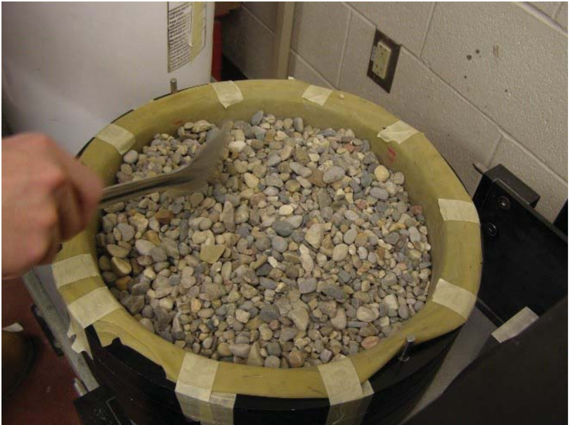
Figure 4.10: Example placement of Pea Gravel in the loose state using small shovel
