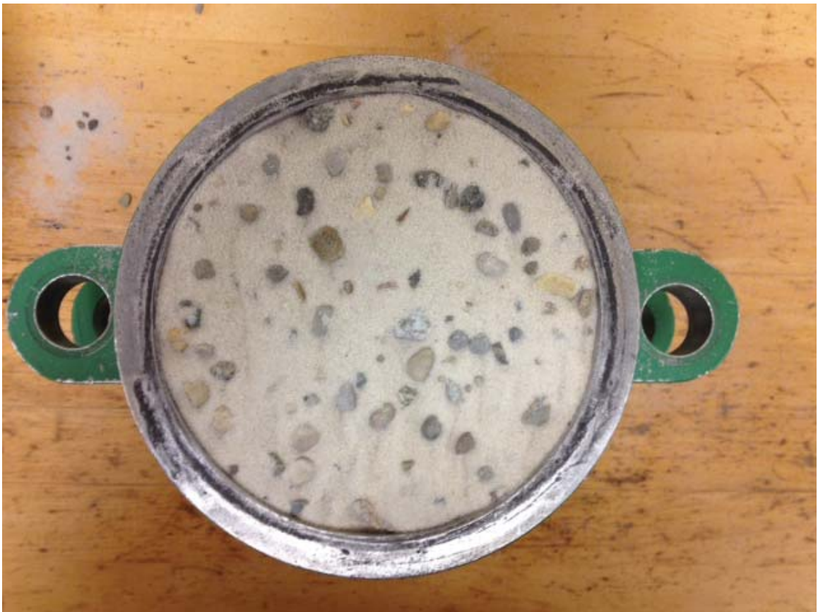
Figure 5.2: 60% Ottawa C109 Sand and 40% Pea Gravel after placement into mold
