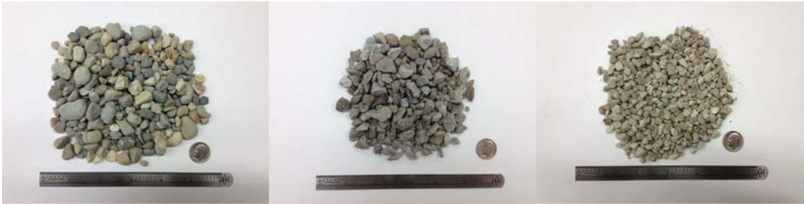
Figure 4.1: Photograph of Pea Gravel, 8 mm Crushed Limestone (CLS8), and 5 mm Crushed Limestone (CLS5)
