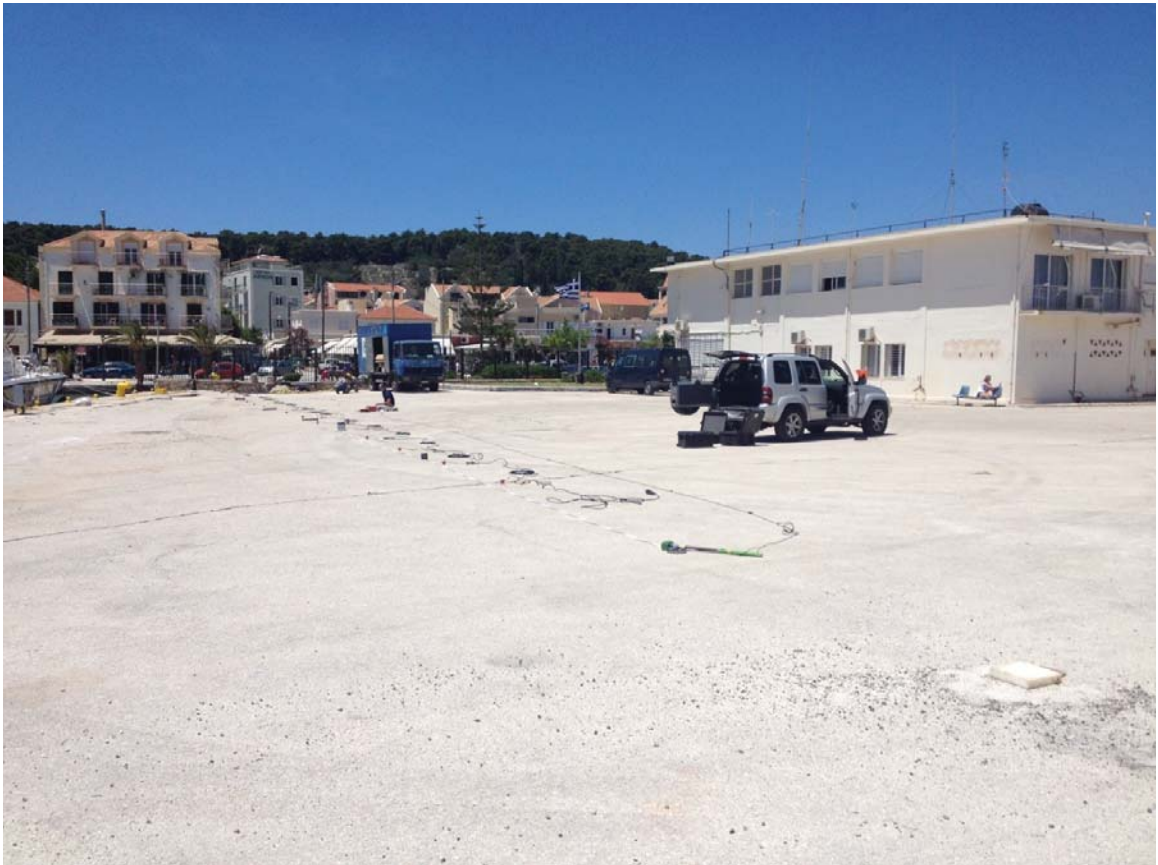
Figure 6.53: MASW setup for V_s measurements at Location 13 with 3 m spacing
