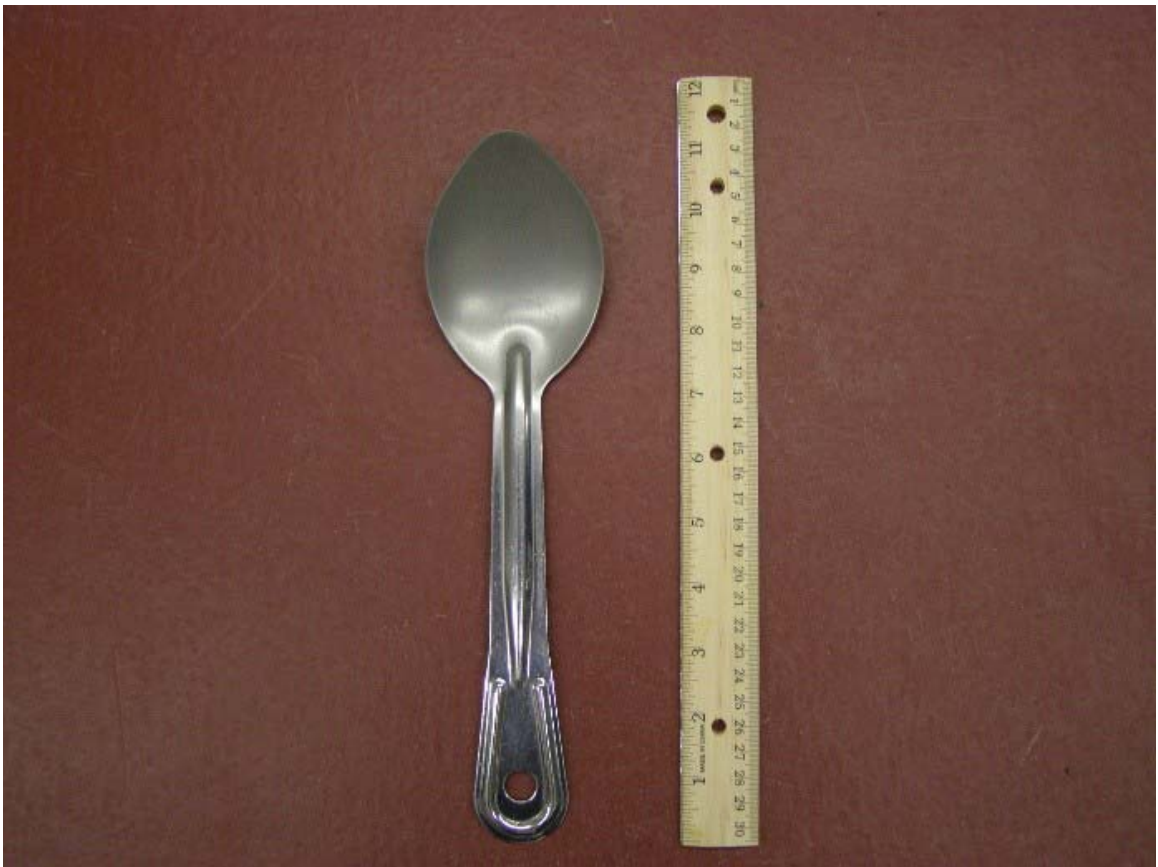
Figure 4.9: Small shovel used for preparation of loose specimens
