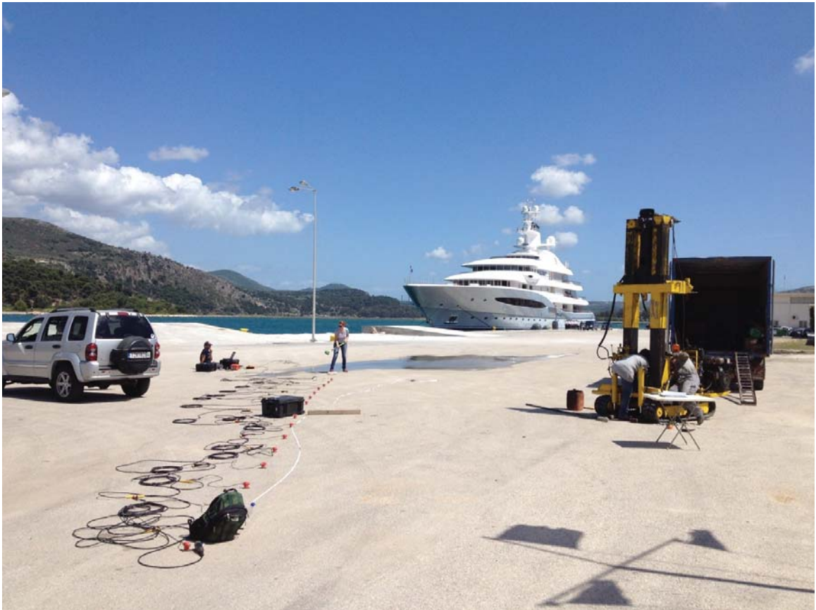
Figure 6.47: MASW setup for V_s measurements at Location 11
