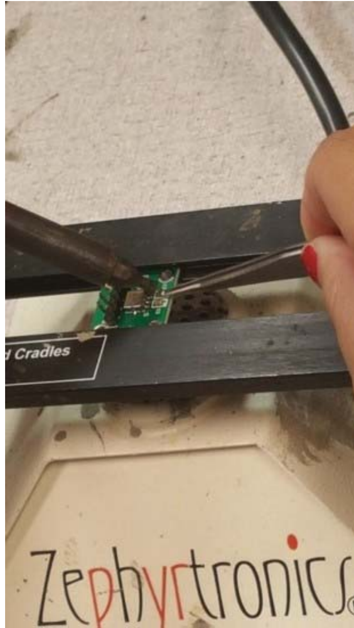
Figure 3.19: Removal of capacitors on ADXL203EB
