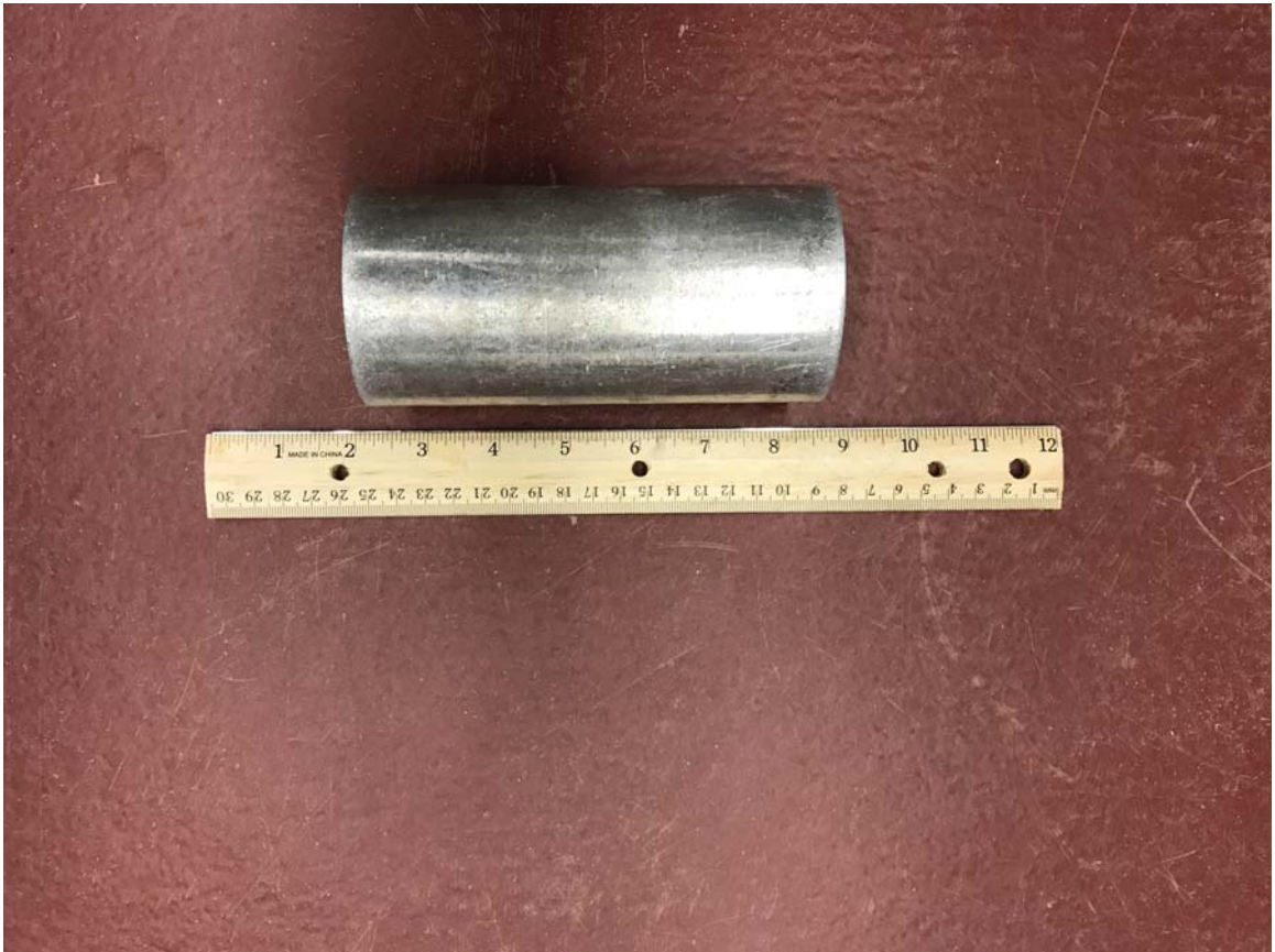
Figure 5.8: Cylinder used for rapid tamping of sand-gravel mixtures
