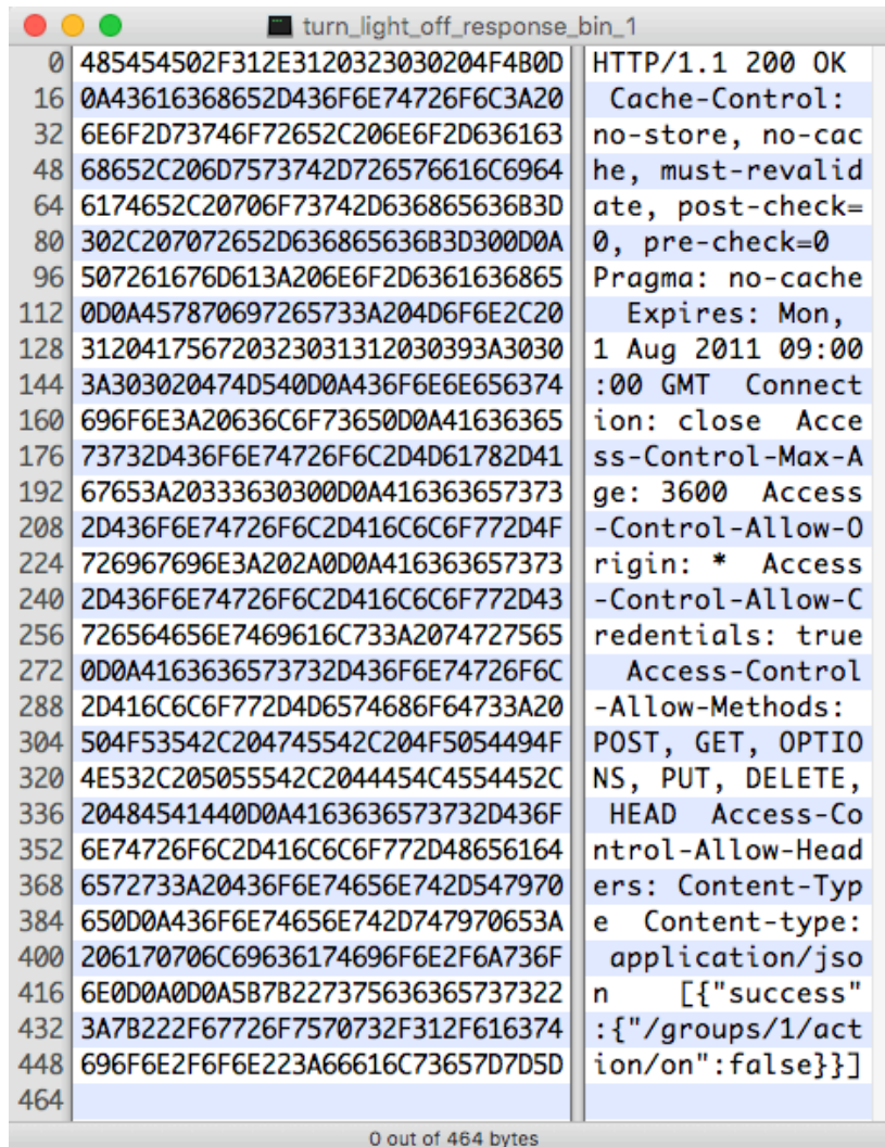
Figure A-11 Turn Smart Light Bulb Off Response Binary Data (From Philips Hue Hub)
