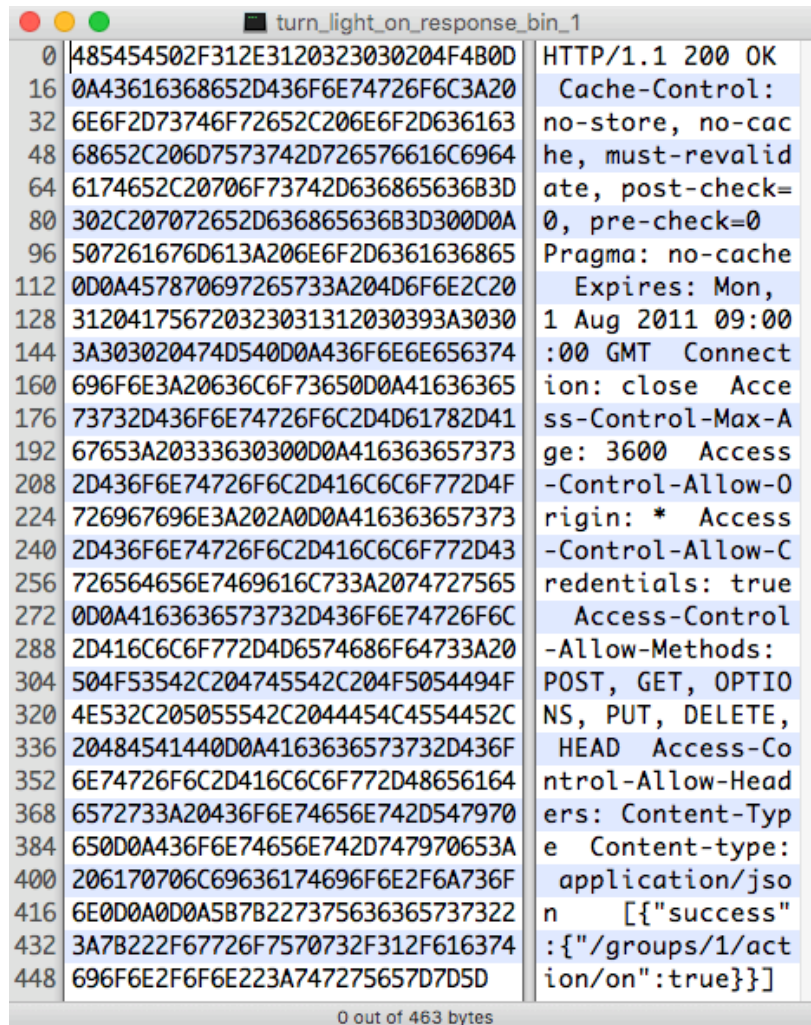
Figure A-7 Turn Smart Light Bulb On Response Binary Data (From Light Bulb)
