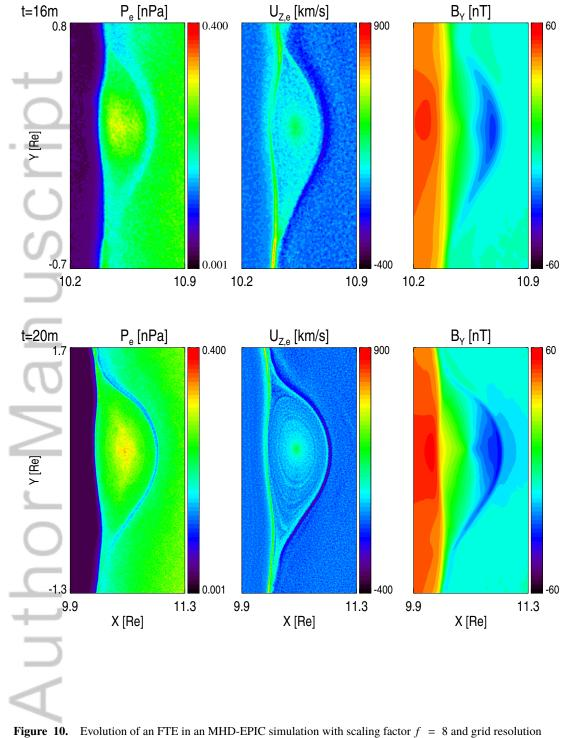
Figure 10. Evolution of an FTE in an MHD-EPIC simulation with scaling factor f = 8 and grid resolution  $\Delta x = 1/128 R_E$ . The electron pressure, the out-of-plane component of the electron velocity and the Y component of the magnetic field are shown for time 16 min (top) and 20 min (bottom). The spatial scales are factor of 2 larger for the later time: the sizes of the panels are  $0.7 \times 1.5 R_E$  and  $1.5 \times 3 R_E$  in the top and bottom rows, respectively.
