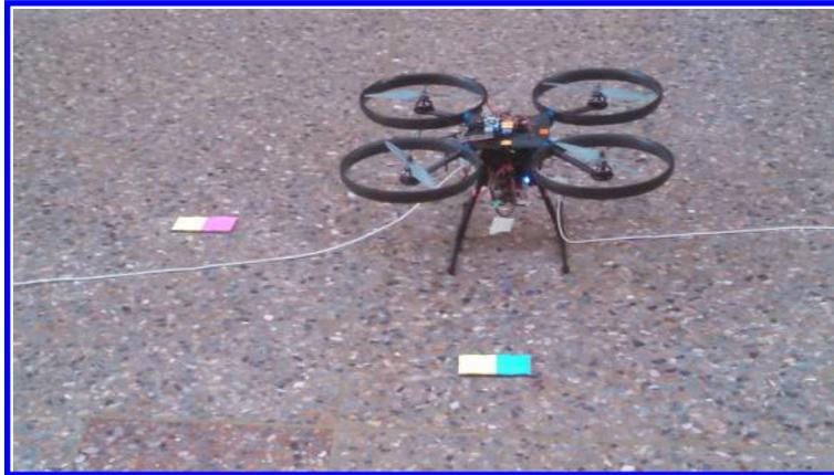
Figure 7. Multicopter with two Pixy color code tags and flight safety tethers.
