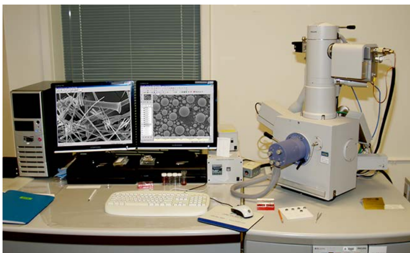
Figure 72 Philips XL30 SEM and EDAX setup
