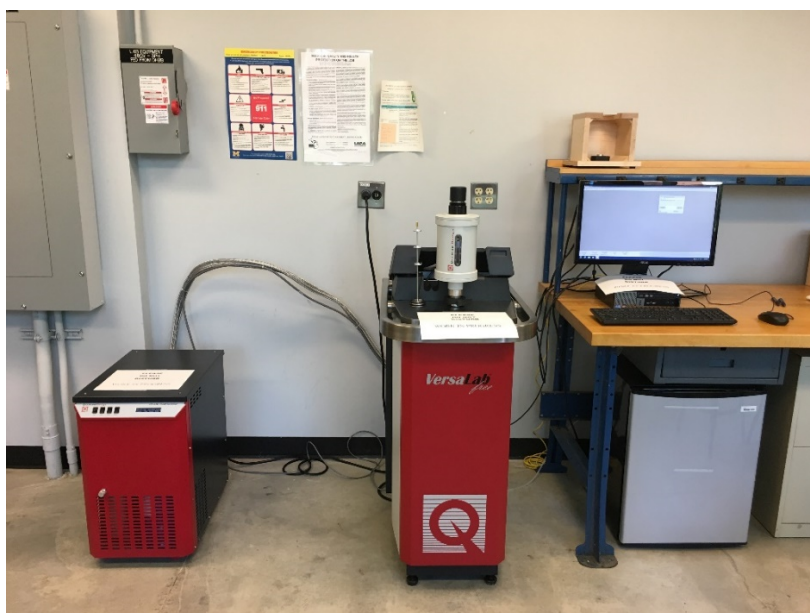
Figure 73 Quantum design's vibrating sample magnetometer setup
