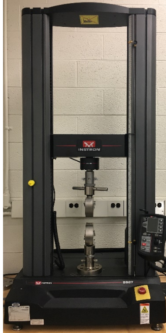
Figure 14 Instron 5597 universal test machine for rates of 0.0025s^{-1} and 0.25s^{-1} .
