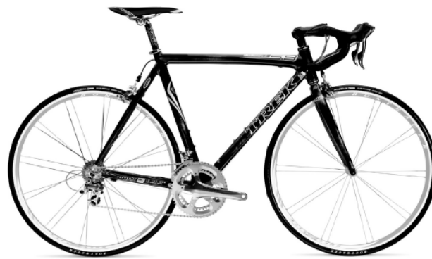
Figure 9 Carbon Fiber Epoxy bicycle frame. [6]
