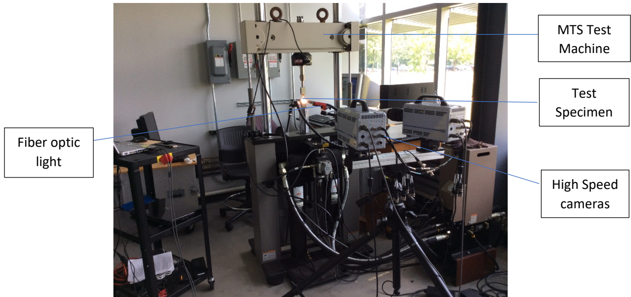
Figure 21 Test setup for high speed tensile testing.
