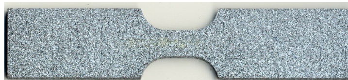
Figure 15 Specimen speckle pattern for DIC analysis.
