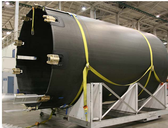
Figure 6 Composite interstage in SpaceX's Falcon 9. [15]
