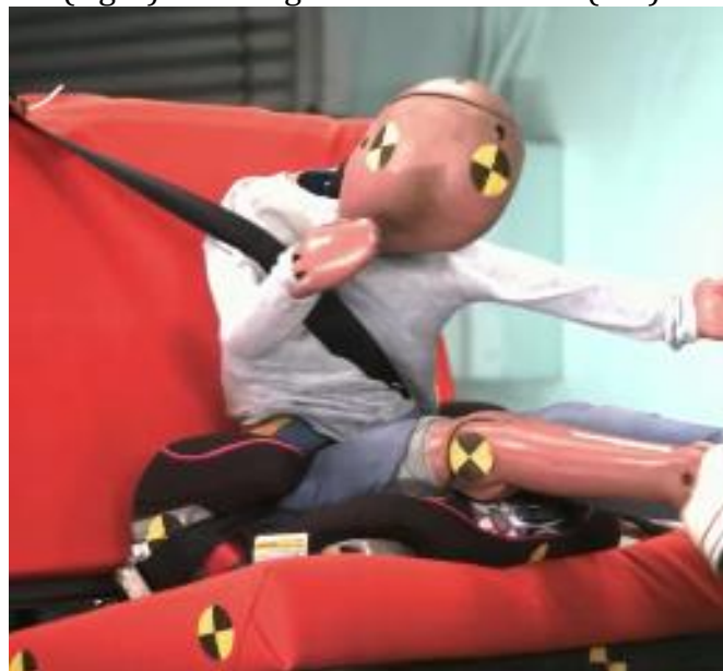
Figure 18. Example of ATD rolling out of the shoulder belt (NT1478).
