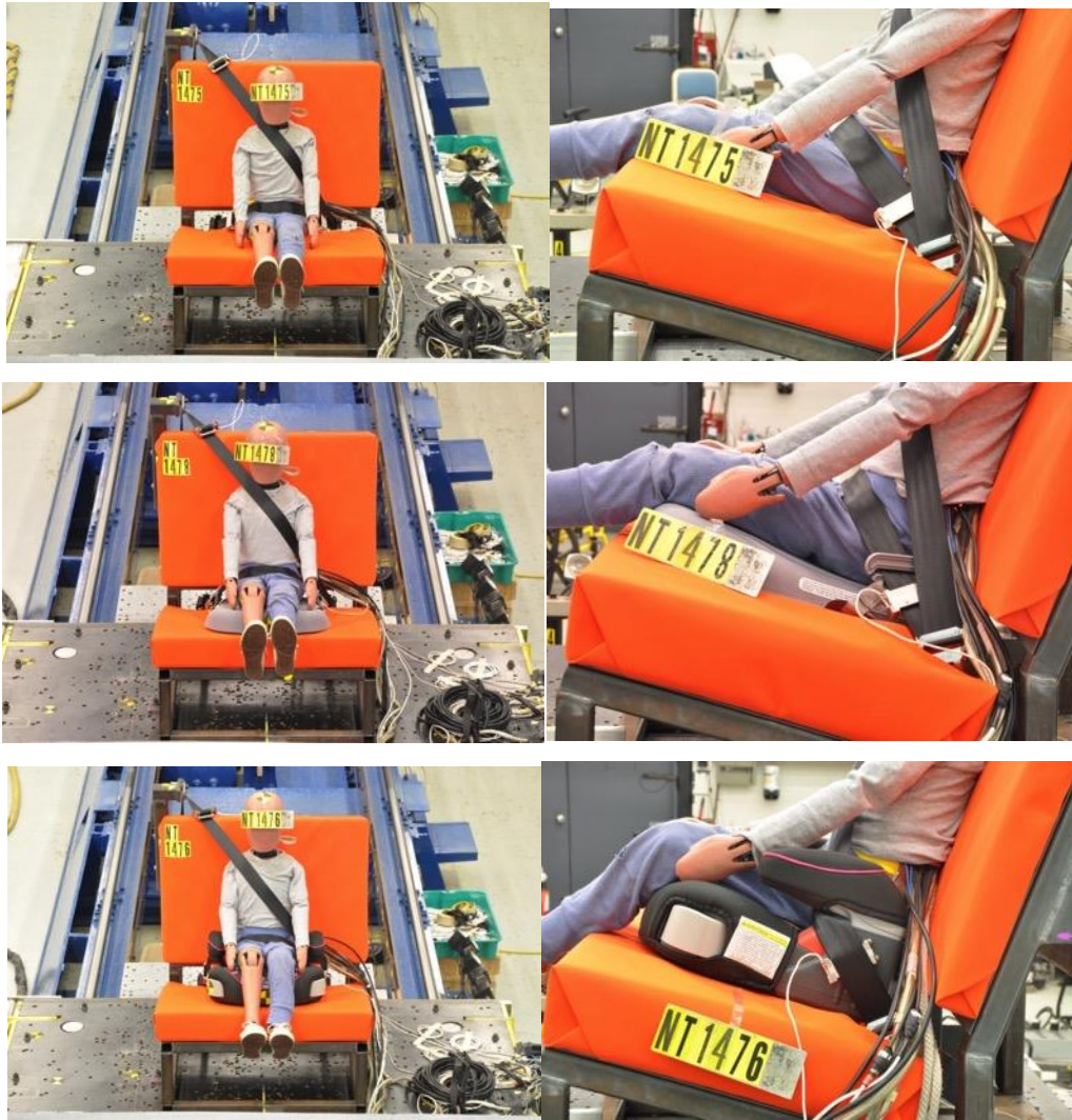
Figure 21. Lap and shoulder belt fit with no booster (top), a 50 mm thick booster (middle) and a 100 mm thick booster (bottom). Shoulder belt scores are -23, -1, and 59.
