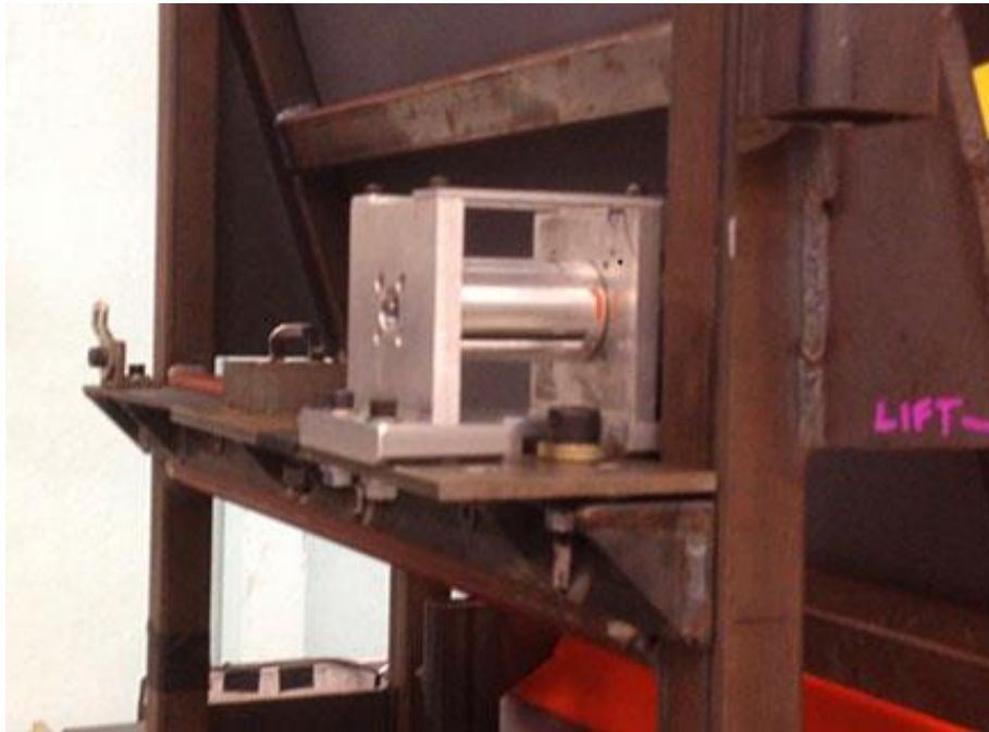
Figure 4. The surrogate shoulder belt retractor.
