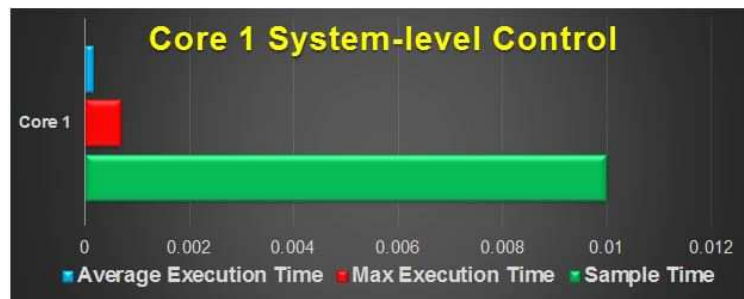
Figure 8.11: Real-time simulation evaluation of system-level controller (core1).
