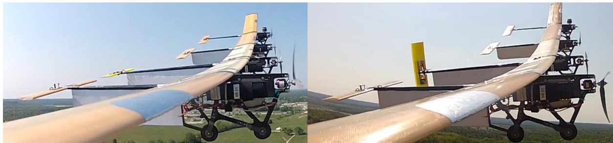
Figure 4.11: X-HALE RRV with center tail in horizontal (l) and vertical (r) configurations during flight.
