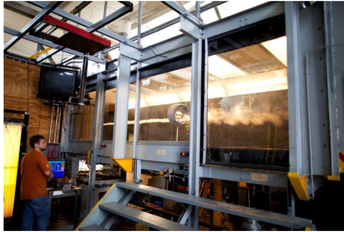
Figure 4.18. External view of test section of the University of Michigan 5x7 wind tunnel
