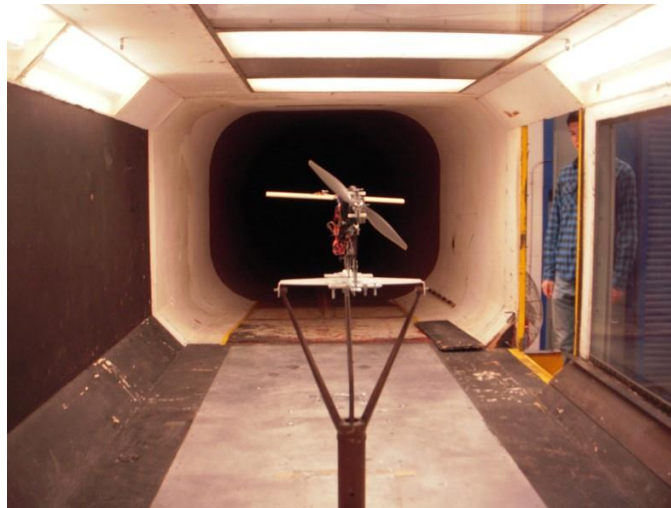
Figure 4.19. Internal view of test section of University of Michigan 5x7 wind tunnel
