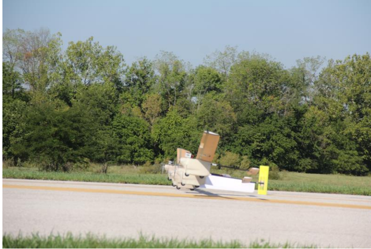
Figure 5.8. X-HALE RRV-6A at takeoff, shown with long center tail, ventral fins, and motor pod fairings
