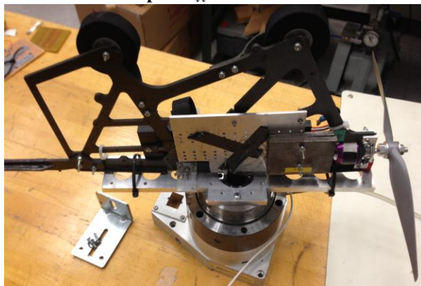
Setup for I_{zz} measurement
