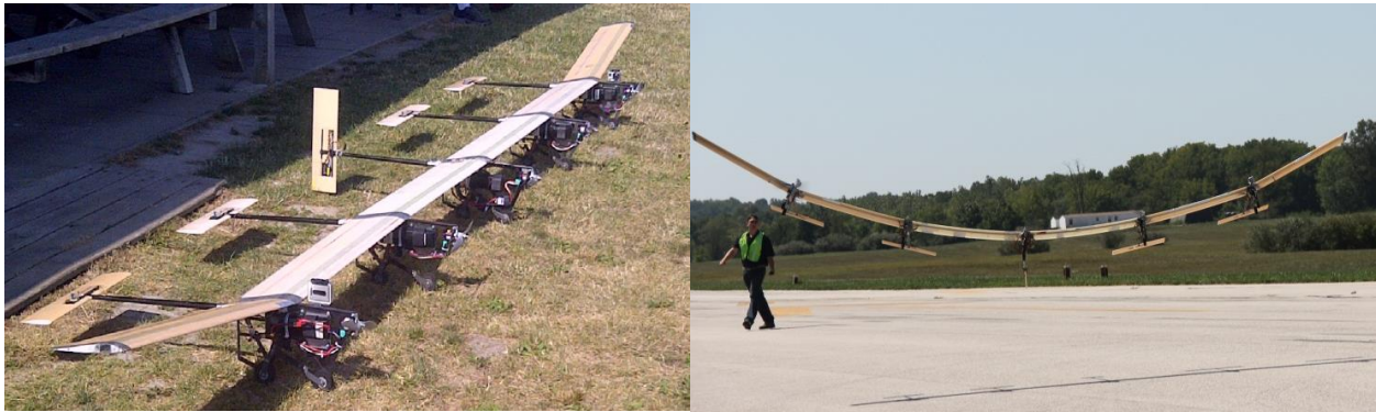
Figure 4.1. The X-HALE unmanned aeroelastic testbed on the ground (l) and at takeoff (r).
