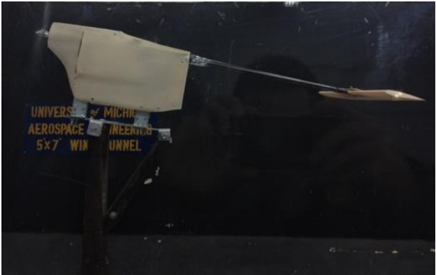
a. Model with no ventral fin at positive angle of attack
