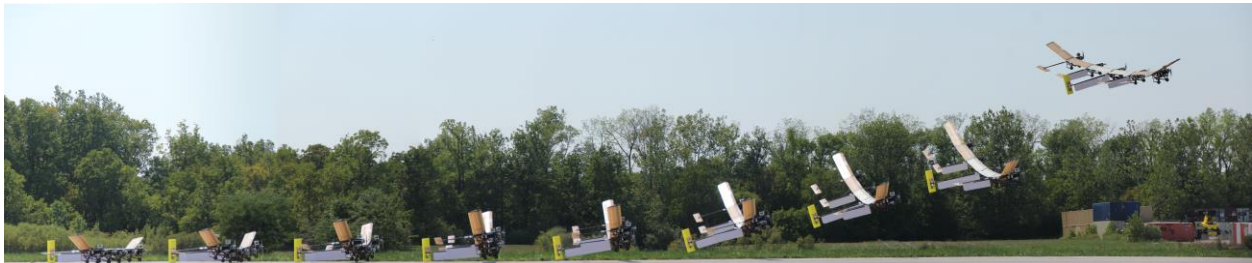
Figure 5.7. RRV-6A during takeoff demonstrating large wing deformation
