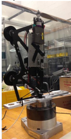
Setup for I_{yy} measurement
