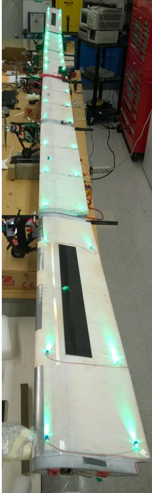
Figure 4.43. X-HALE ATV-B LED markers for the stereovision wing shape measurement system
