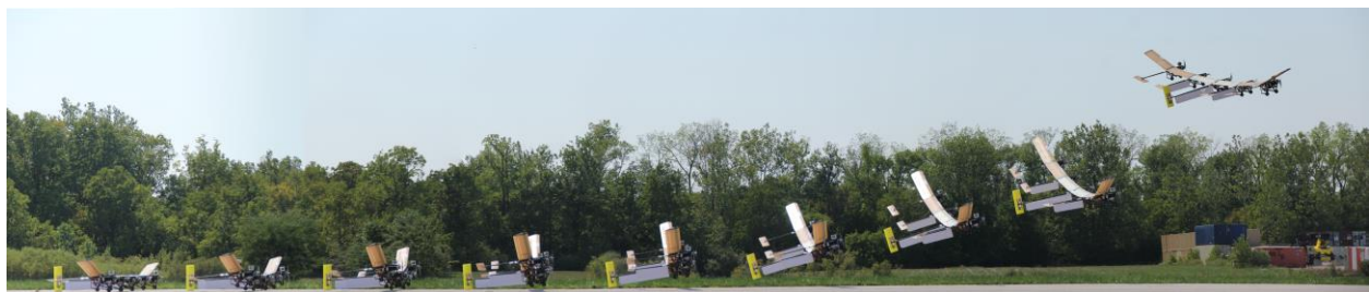
Figure 4.38: X-HALE RRV-6A with elongated center tail and ventral fins showing large wing deflections during takeoff
