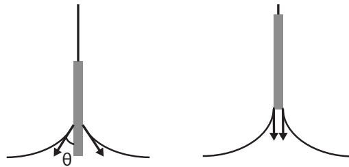
Figure 2.8: Closeup of strip. Arrows depict direction of surface tension force. At pinch-off the forces are parallel to the strip.
