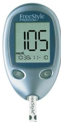
Figure 1.1: A glucose meter that allows diabetics to monitor the sugar content of their blood. A drop of blood is obtained with a lancet and placed on a wicking strip that is analyzed by the meter.
