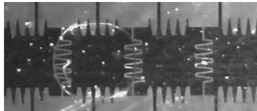
Figure 1.18: Picture of EWOD-based droplet actuation device as seen from above, from Pollack et al. [2000]. The top electrode is made of a transparent material, indium-tin-oxide (ITO). The light gray areas are metal electrodes. The transparent water droplet is on the left, delineated by its glint. The electrode pitch is 1.5 mm
