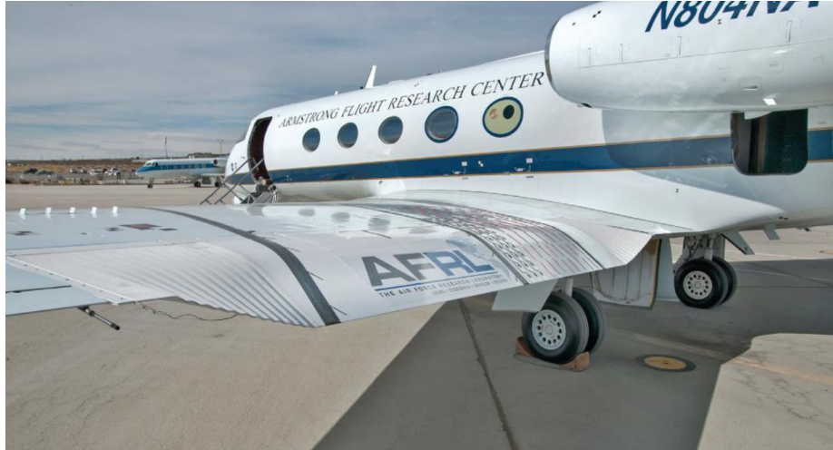
Figure 1.5: The 19-foot ACTE device installed on the testbed aircraft used in flight tests in 2014, deflected at 20^\circ [43].
