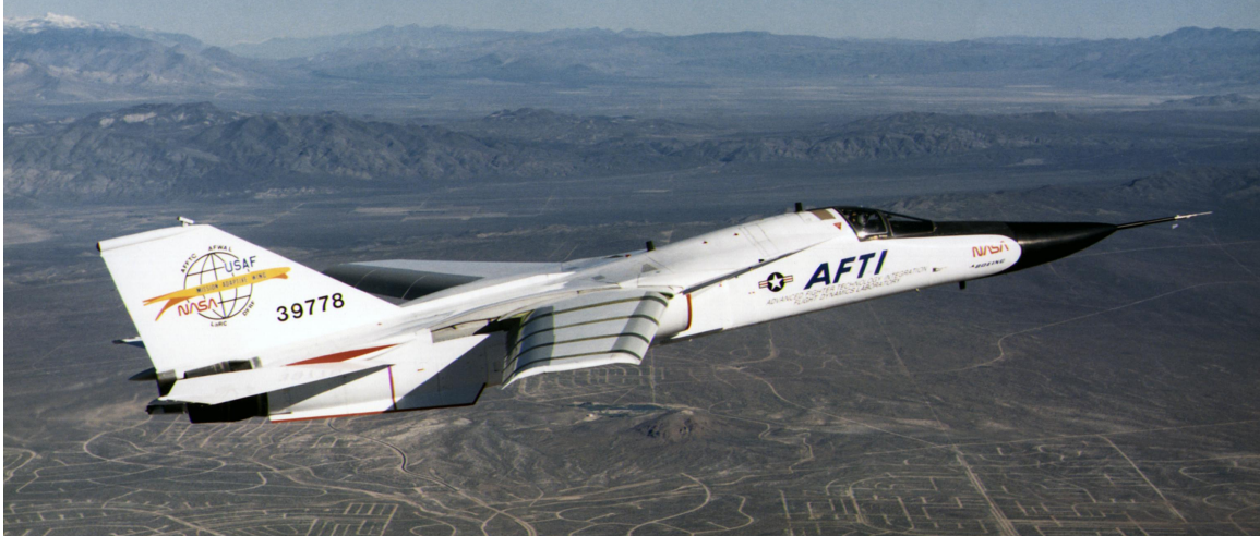
Figure 1.3: The retrofit wings on the AFTI test aircraft included supercritical MAW devices on the leading and trailing edges.
