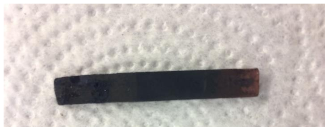
Figure 4-9 The cathode after the \text{Cu}_{1.5}\text{PMo}_{12}\text{O}_{40} charge/discharge, the brown copper could be seen clearly on the right side in the picture
