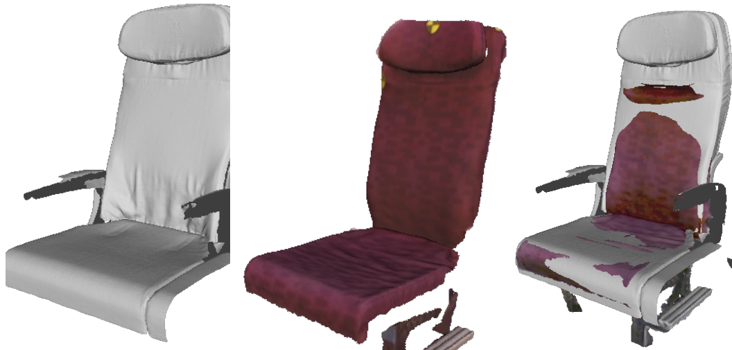
Figure 6. Scan of aircraft seat (left), the mockup seat (middle), and overlaid (right).
