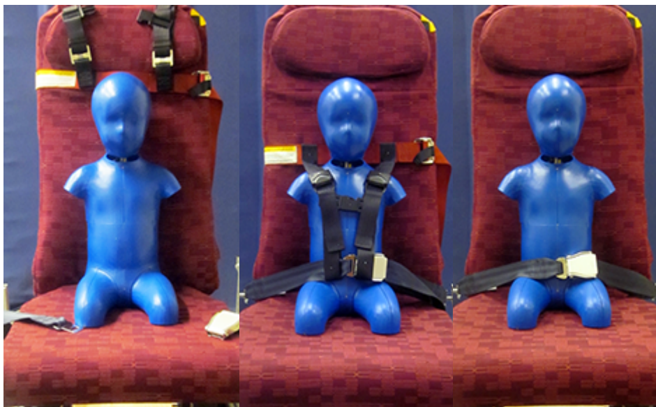
Figure 27. Photos of the manikin with a harness and lap belt.
