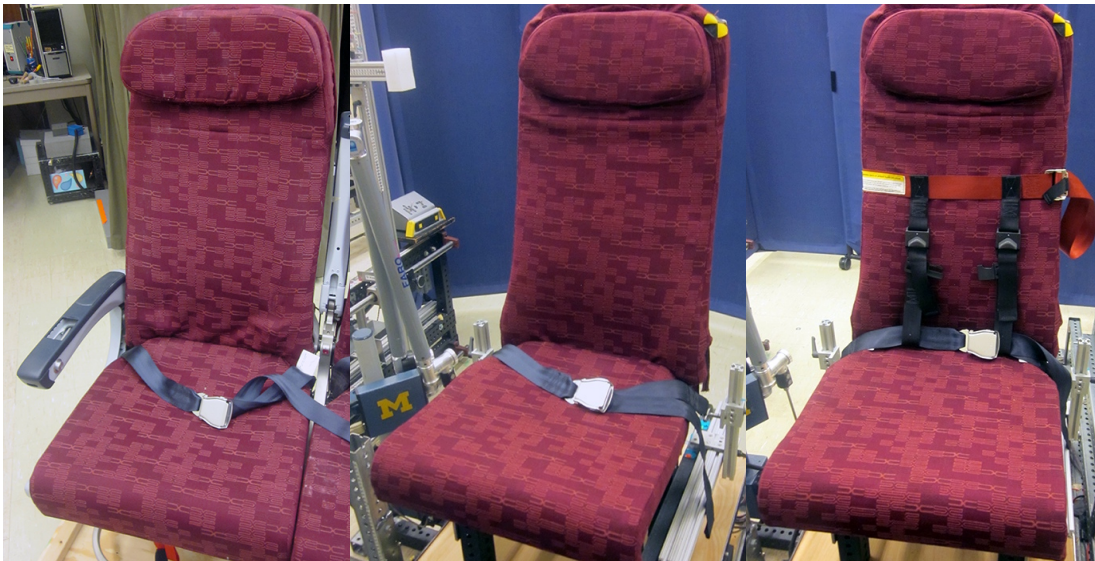
Figure 9. Aircraft seat as manufactured on aluminum frame (left), aircraft seat cushions mounted on laboratory frame with lap belt (center) and lap belt plus CARES harness (right).
