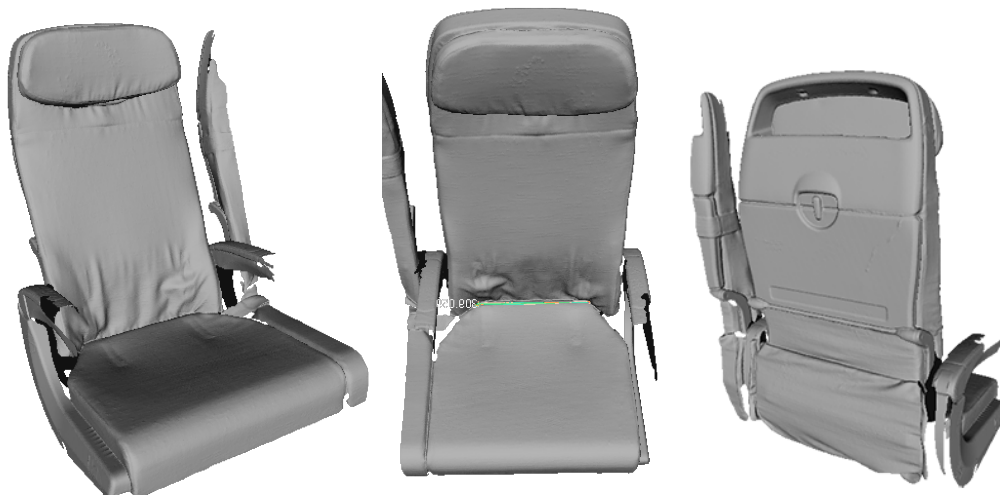
Figure 4. Surface scans of an aircraft seat.
