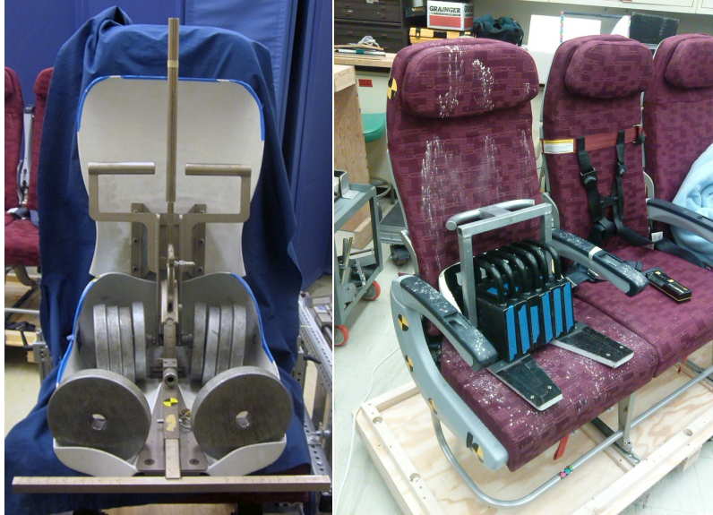
Figure 5. J826 H-point machine (left) and Seat Index Point Tool (right) used to characterize seat geometry.
