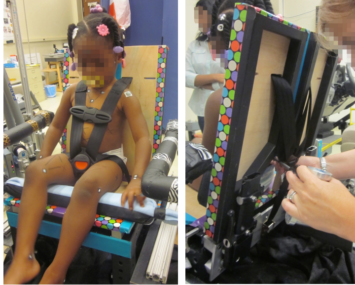
Figure 16. Child sitting in the hardseat (left) and an investigator digitizing the child's spine and pelvis through the opening in the back of the seat (right)
