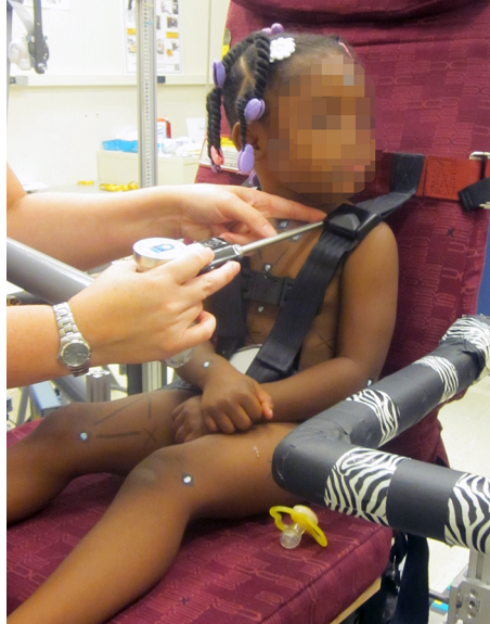
Figure 11. Investigator digitizing points on restraint system
