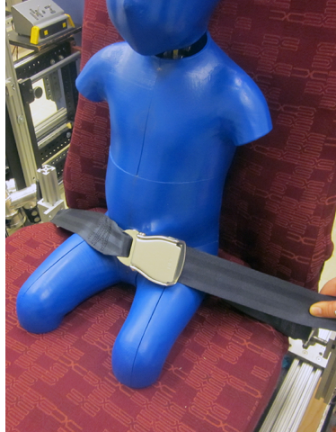
Figure C3. Investigator applying lap belt
