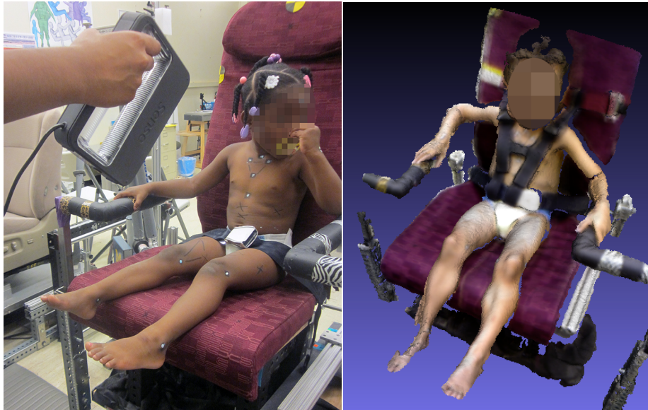
Figure 24. Participants were also scanned while in aircraft seat using a Sense hand-held scanner.
