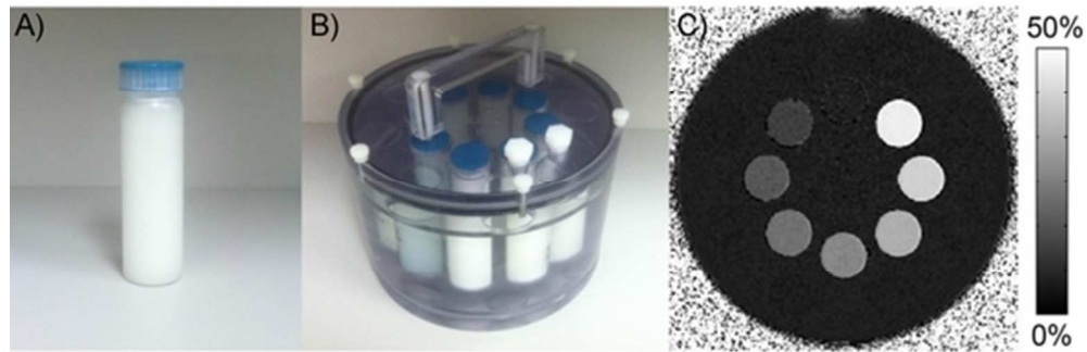
(A) Vial consisting of a predetermined proton-density fat fraction (PDFF). (B) Multiple vials can be scanned simultaneously by placing them in a phantom holder that is filled with deionized water (128). (C) The PDFF for each of the vials can be estimated using MRI. In this example, the PDFF values are (beginning at 12 o'clock position and moving counterclockwise) 0 %, 5 %, 10 %, 15 %, 20 %, 30 %, 40 %, and 50 %.
