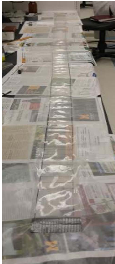
Figure 3. Photograph of a long PS embedded PVA film produced by Step 1.
