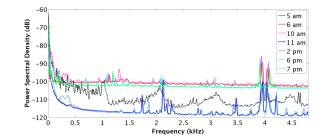
Figure 3. Power spectral density (PSD) of the ambient noise recorded in the pipe at different times of the day.
