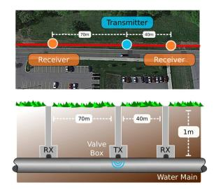
Figure 1. Field experiment for testing the Awa system. Signals are sent by a transmitting (TX) node and recorded by two receiving (RX) nodes.
