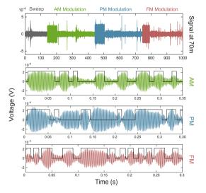
**Figure 6.** Fully measured waveform at 40 m of the entire signal (top figure), including the sweep and each modulation scheme, and segments of 500 Hz modulated signals (bottom three figures). Black, solid lines indicate the bits that were transmitted.
