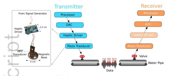
Figure 2. Node and system architecture. Each node switches between transmitter and receiver mode. In transmitter mode, a digitalto-analog converter (DAC) is used to drive the transducer. In receiver mode, the haptic driver is bypassed and an analog-to-digital (ADC) converter is used to directly measure the vibrations from the receiving piezo.
