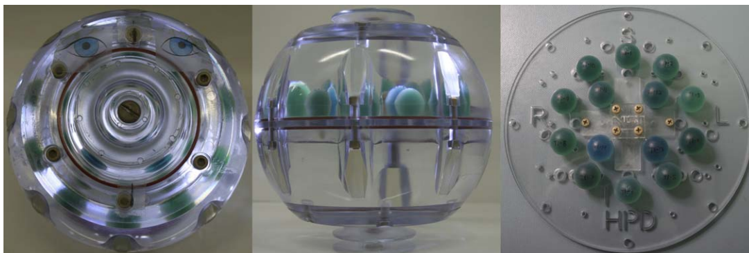
FIG. 1. (left) View of the NIST T_1 phantom from the top. Phantom positioning mimics the positioning of a patient lying head-first, supine on the MRI table (eye decals facing up, toward the scanner bore), so that the central plate is parallel to the coronal imaging plane. (center) View of the T_1 phantom from the side. (right) Central plate of the NIST T_1 phantom demonstrating positioning of the 14 samples (S1–S14) of \text{NiCl}_2 solution, with T_1 ranging from 22 to 2033 ms in descending order, determined by NMR spectroscopy at 1.5 and 3 T (Supporting Table S3).
