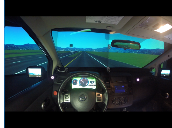
Figure 1: Video screenshot of driving conditions taken from a first person perspective driving view in a high-fidelity vehicle simulator
