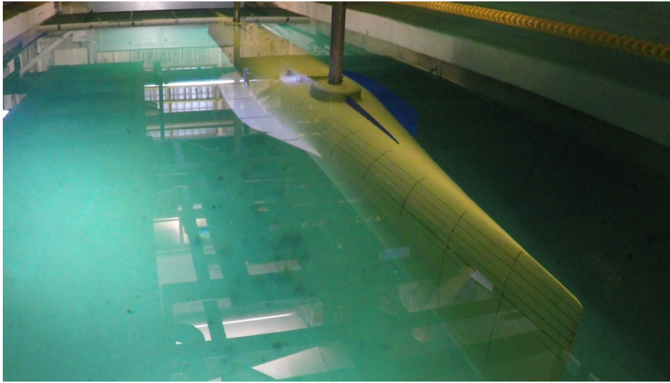
Figure 4: CSS Hunley model at static completely submerged condition (test cases 3 and 4)
