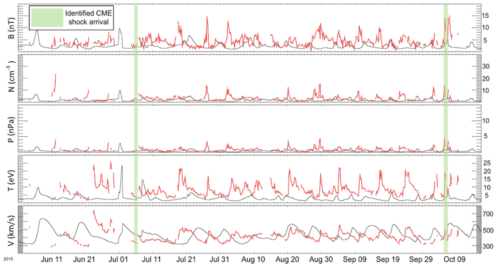
Figure 9: Identified CME shock arrival times (light green) from June to October 2015 for the extended run as observed by MAVEN (red) and predicted by WSA-ENLIL+Cone (black)
