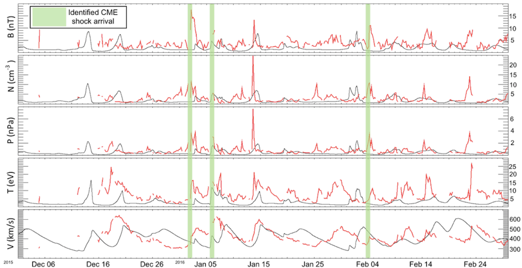
Figure 3: Identified CME shock arrival times depicted in light green from the detailed simulation (December 2015 to March 2016). MAVEN's observations are depicted in red, while WSA-ENLIL+Cone dataset is in black.
